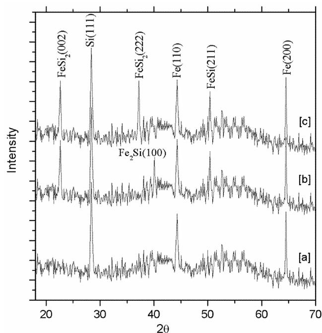
**Figure 1.** XRD of (a) as deposited sample, (b) irradiated sample with 120 MeV  $Au^{+9}$  ions at a dose of  $5 \times 10^{12}$  ions/cm<sup>2</sup> and (c) irradiated sample with 120 MeV  $Au^{+9}$  ions at a dose of  $5 \times 10^{13}$  ions/cm<sup>2</sup>.
