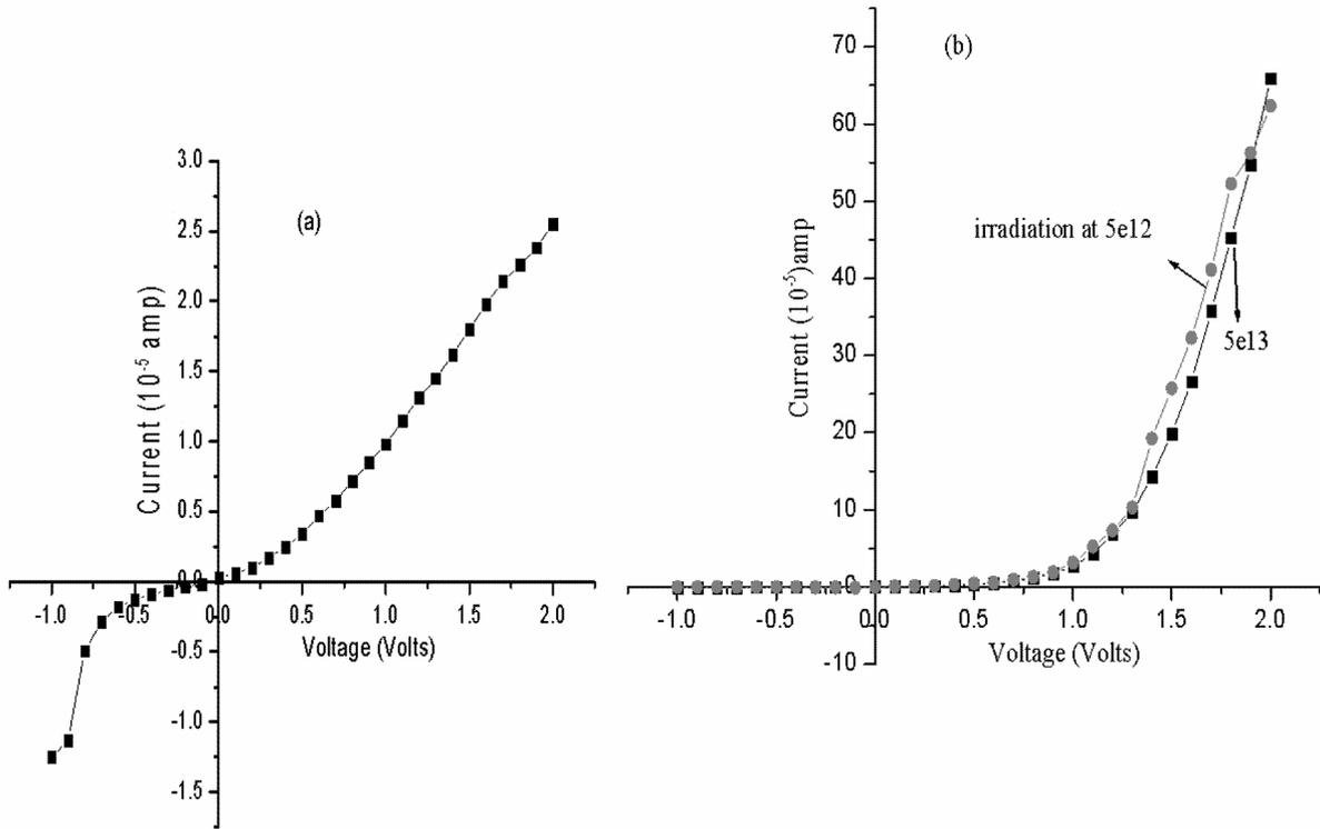
**Figure 2.**  $I$ - $V$  curve for (a) pristine sample and (b) irradiated sample.
