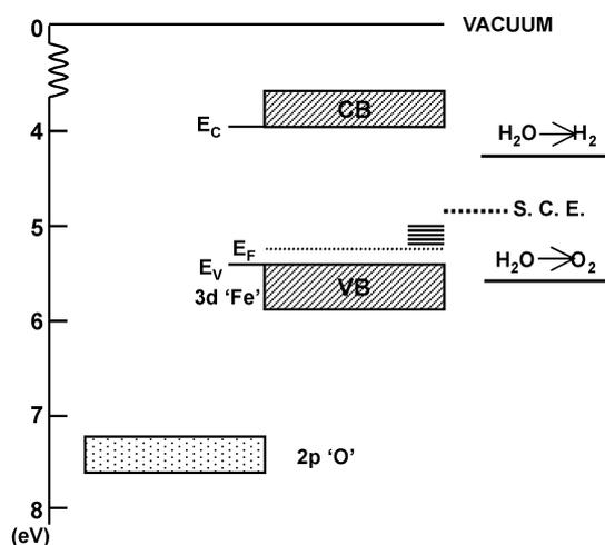
Figure 1. Energy band diagram of CuO.
