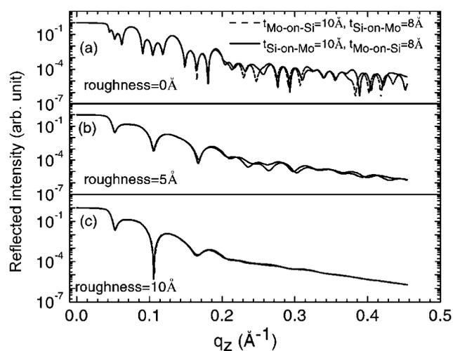
**Figure 5.** The simulation spectra of the effect of asymmetry interlayer thickness on reflectivity profile of  $N = 4$  MLs for different roughness values.
