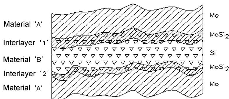
**Figure 2.** A schematic diagram of real multilayer structure with interlayer. The four-layer model shows imperfect boundaries and interlayer in between two pure Mo and Si layers.
