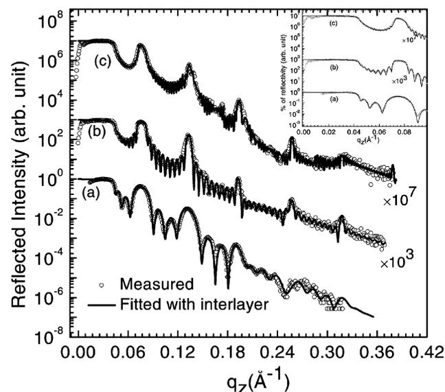
**Figure 6.** The Mo/Si MLs measured reflectivity data of figure 1 is re-plotted along with four-layer model fitting. Open circles represent the measured data. The continuous line shows calculated spectra with four-layer model: (a) for MLs with  $N = 4$ , (b) for MLs with  $N = 10$  and (c) for MLs with  $N = 20$ . The inset shows the distinct Kiessig oscillations up to 1st Bragg peak.
