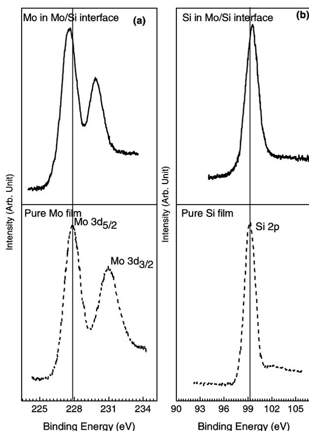
**Figure 8.** XPS spectra using Al  $K_{\alpha}$  source. (a) Mo  $3d$  core level spectra recorded for pure Mo film (dash) and Mo at interfaces of Mo/Si MLs and (b) Si  $2p$  core level spectra recorded for pure Si film (dash) and Si at interfaces of Mo/Si MLs.
