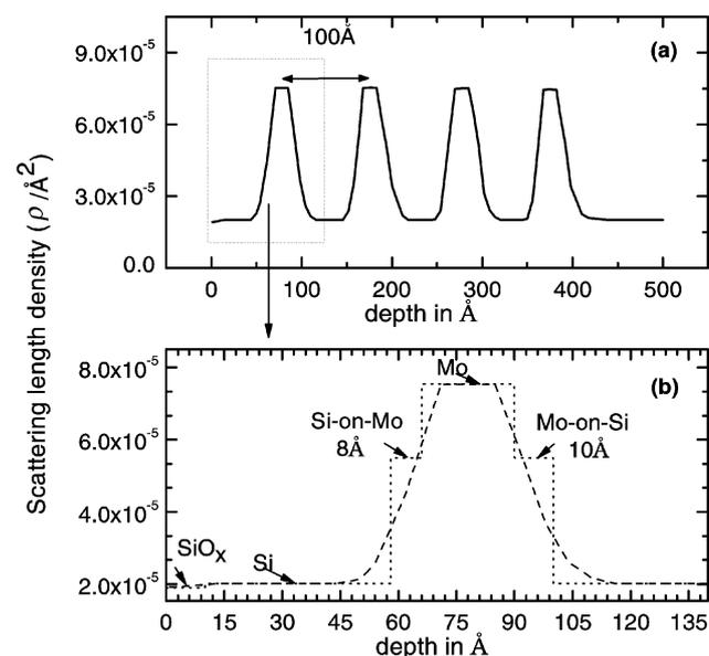
**Figure 7.** Scattering length density profile obtained after fitting of experimental data using interlayer. (a) Maxima and minima correspond to layers of pure Mo and Si, respectively. In between are the interface region arising from the formation of silicide interlayer and layer roughness and (b) the dashed (----) line represents actual profile used for fitting assuming interlayers with Gaussian roughness. The dotted (.....) line represents the profile without Gaussian roughness.
