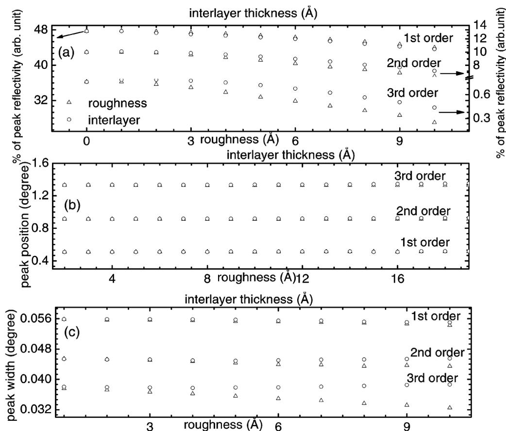
**Figure 4.** The simulation studies of the effect of roughness (open triangles) and interlayer (open circles) on higher order Bragg's peak for  $N = 4$  MLs. (a) Effect on higher order Bragg peak reflectivity, (b) effect on higher order Bragg peak position and (c) effect on higher order Bragg peak width.
