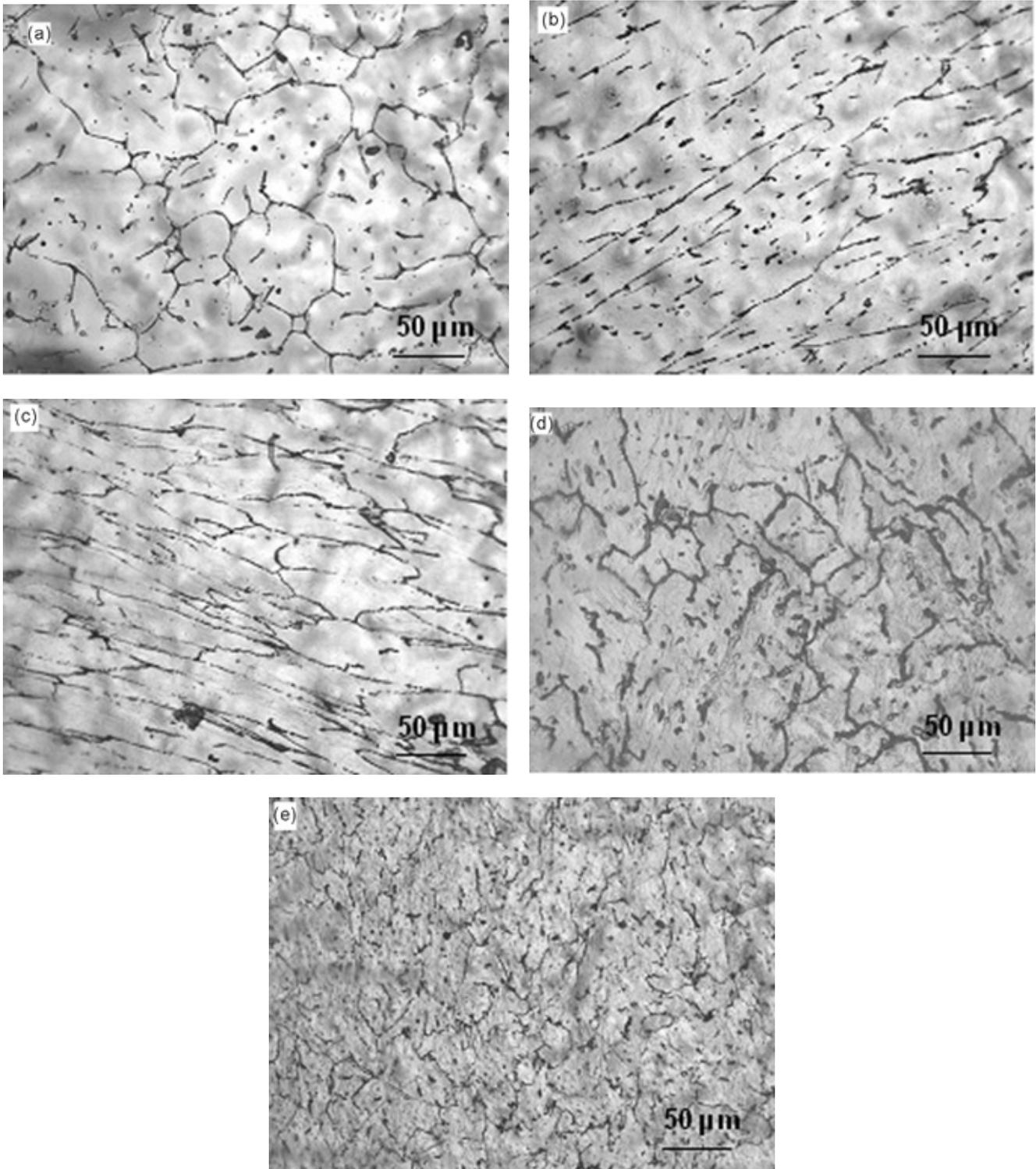
**Figure 4.** Optical microstructures of 99.5% pure aluminium: (a) unpressed, (b) after first pass, (c) after second pass, (d) after third pass and (e) after fourth pass.
