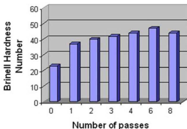
**Figure 7.** Variation of hardness with the number of passes in 99.5% pure aluminium.
