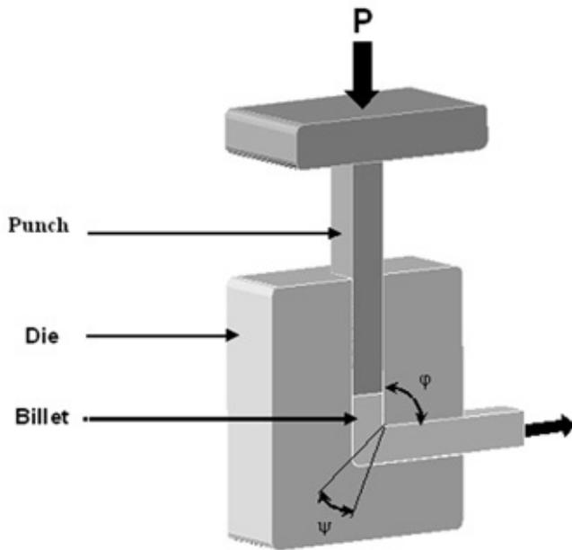
**Figure 1.** Schematic of ECAP.
