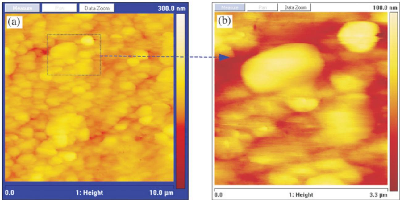
**Figure 5.** AFM microstructures of 99.5% pure aluminium after 8 passes.
