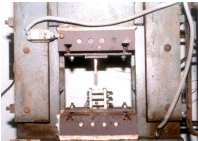
**Figure 2.** ECAP die assembly fitted to the hydraulic press.
