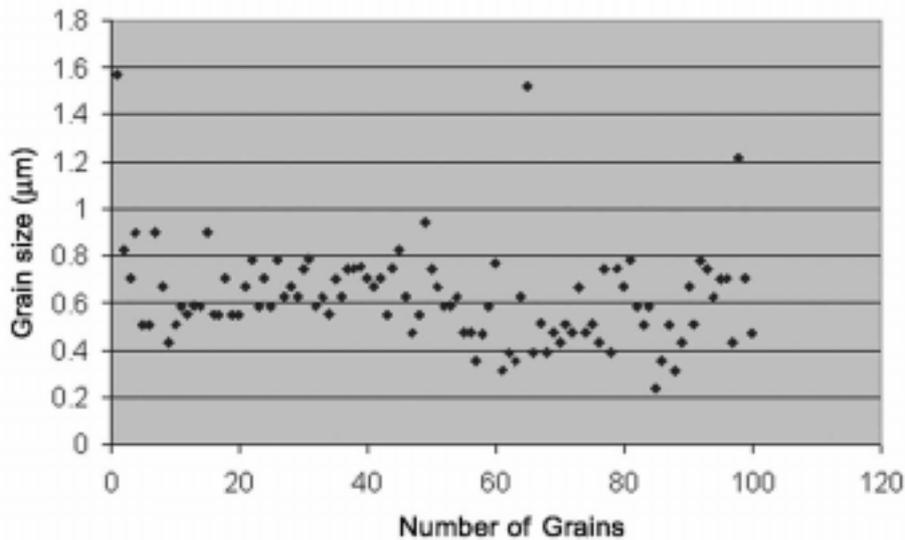
**Figure 6.** Grain size distributions of 99.5% pure aluminium after 8 passes.
