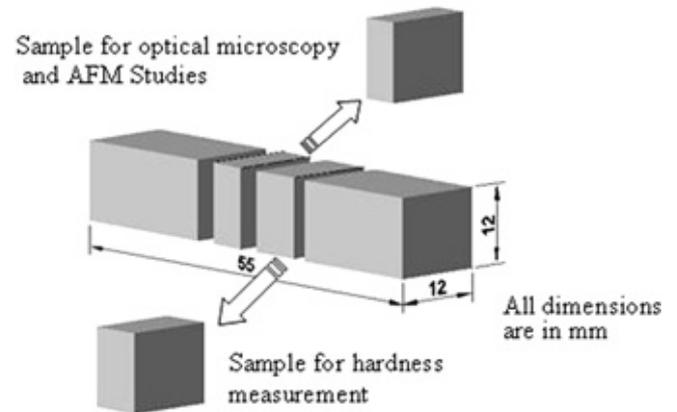
**Figure 3.** Location of specimens for AFM, optical and hardness evaluation.
