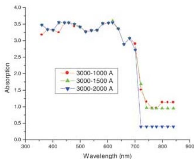
**Figure 2.** Wavelength vs absorption of ion beam irradiated Al–Sb bilayer thin films of thicknesses, 3000–1000 Å, 3000–1500 Å and 3000–2000 Å.
