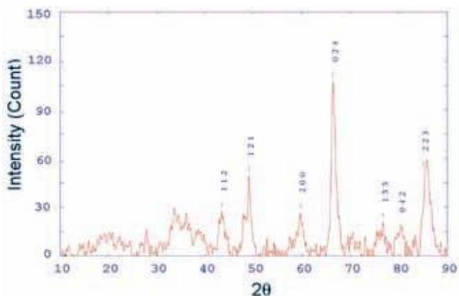
**Figure 8.** X-ray diffraction pattern of ion irradiated Al–Sb bilayer thin film of thickness, 3000–1500 Å.
