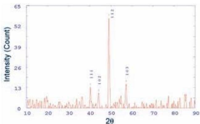
**Figure 7.** X-ray diffraction pattern of as deposited Al–Sb bilayer thin film of thickness, 3000–1500 Å.
