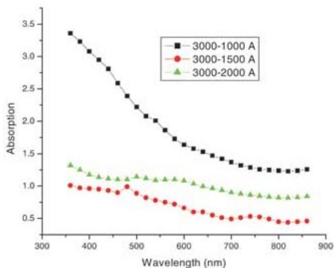
**Figure 1.** Wavelength vs absorption of as deposited Al–Sb bilayer thin films of thicknesses, 3000–1000 Å, 3000–1500 Å and 3000–2000 Å.
