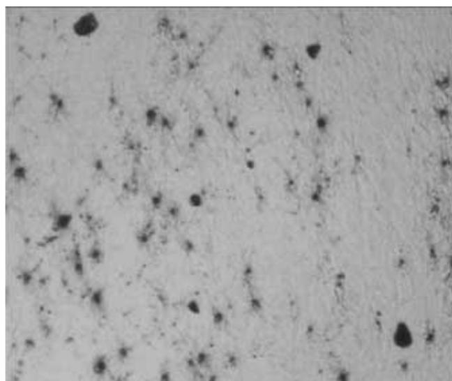
**Figure 9.** Microphotograph of as deposited Al–Sb bilayer thin film of thickness, 3000–1500 Å.
