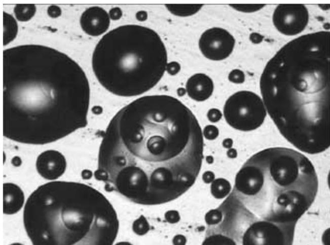
**Figure 10.** Microphotograph of ion irradiated Al-Sb bilayer thin film of thickness, 3000–1500 Å.
