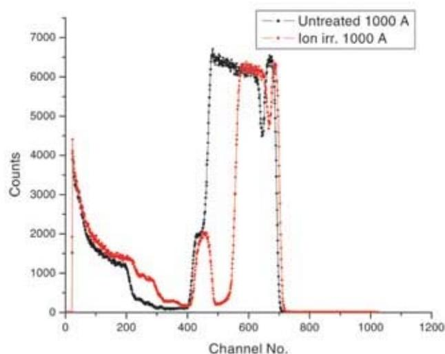
**Figure 4.** Rutherford backscattering spectra of as deposited and ion beam irradiated Al-Sb thin film of thickness, 3000–1000 Å.
