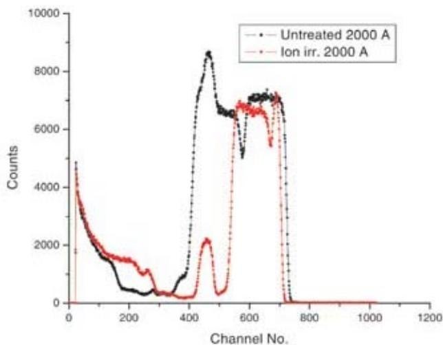
**Figure 6.** Rutherford backscattering spectra of as deposited and ion beam irradiated Al–Sb thin film of thickness, 3000–2000 Å.
