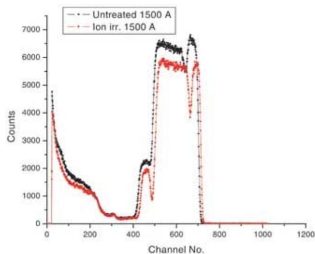
**Figure 5.** Rutherford backscattering spectra of as deposited and ion beam irradiated Al-Sb thin film of thickness, 3000–1500 Å.
