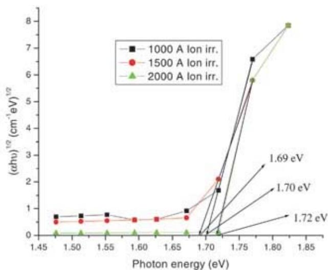
**Figure 3.** Photon energy vs  $(\alpha h\nu)^{1/2}$  of ion beam irradiated Al-Sb thin films for thicknesses, 3000–1000 Å, 3000–1500 Å and 3000–2000 Å.
