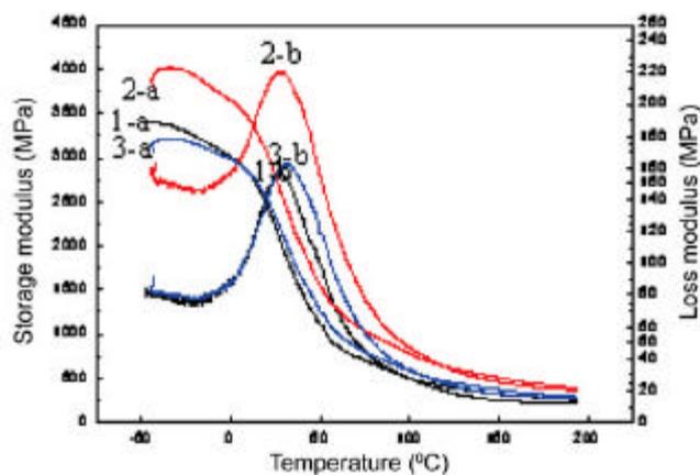
**Figure 5.** Plots of storage modulus and loss modulus versus temperature of nylon 66 and nanocomposites.
