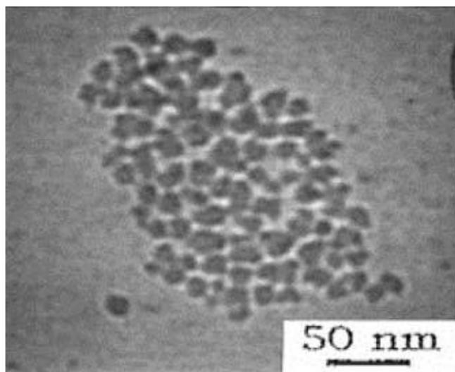
Figure 2. TEM image of SiO<sub>2</sub> nanoparticles.
