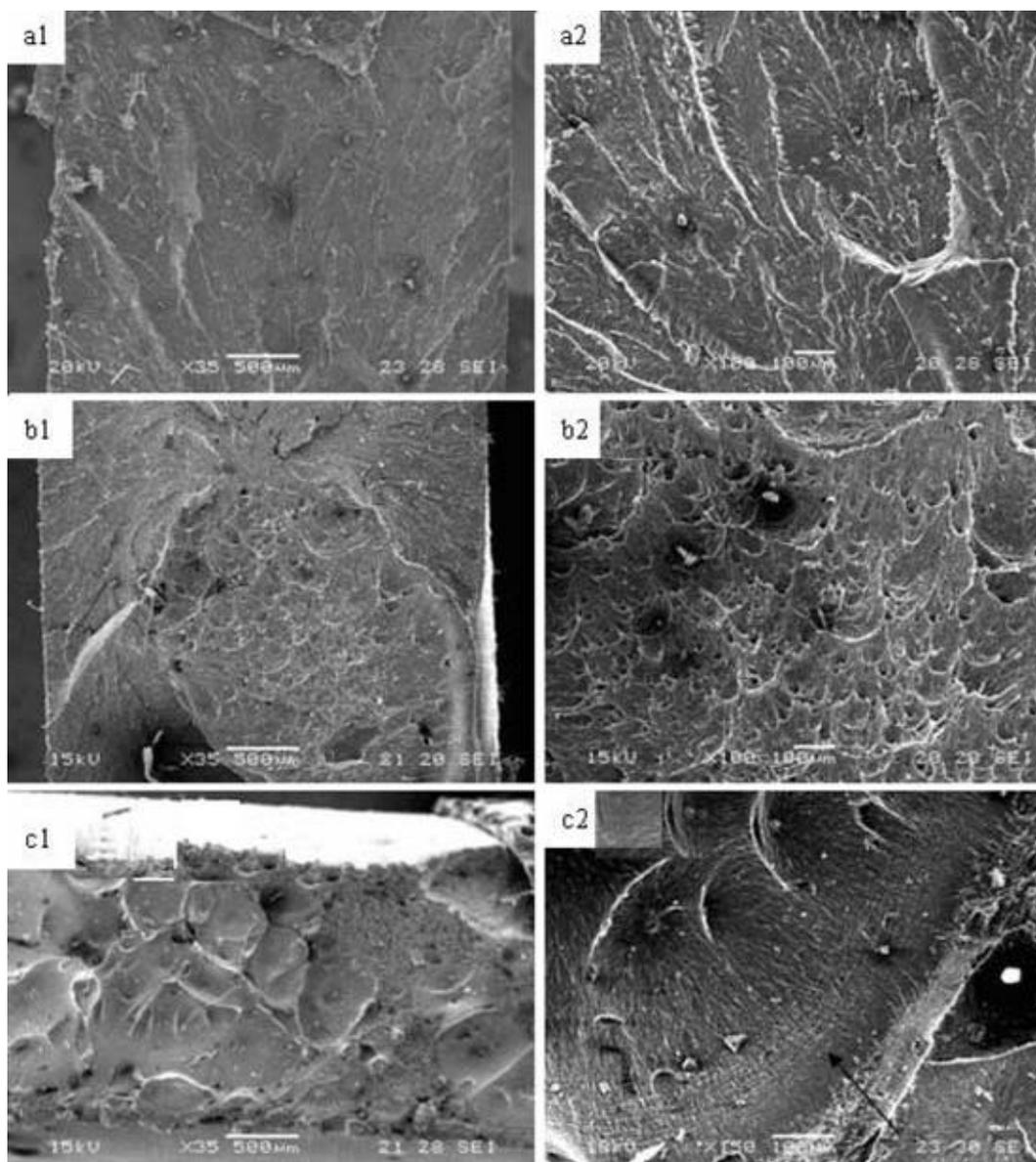
**Figure 3.** The tensile fracture of PA 66 and its nanocomposites.
