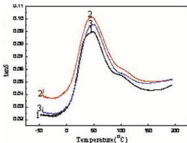
**Figure 6.** Plots of  $\tan \delta$  vs temperature of nylon 66 and nanocomposites.
