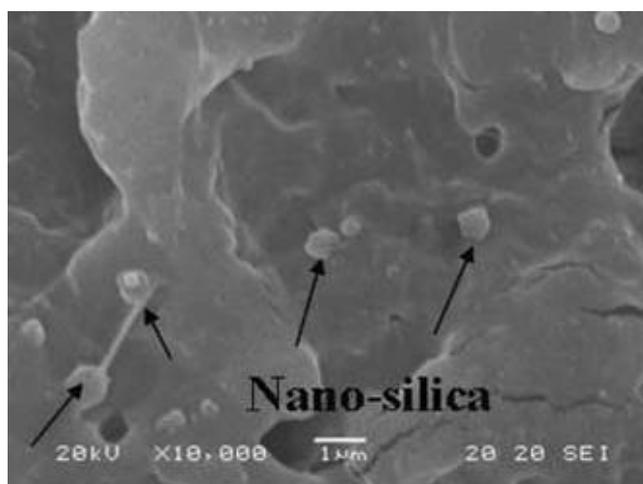
**Figure 7.** The tensile fracture at a higher magnification of PNSC-3.
