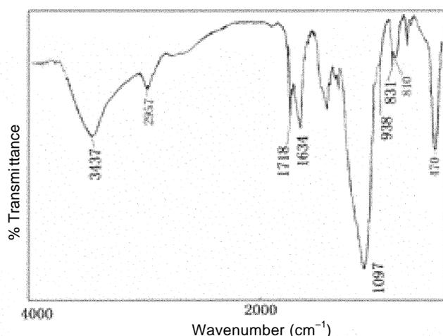
Figure 1. FT-IR spectra of SiO<sub>2</sub> nanoparticles.
