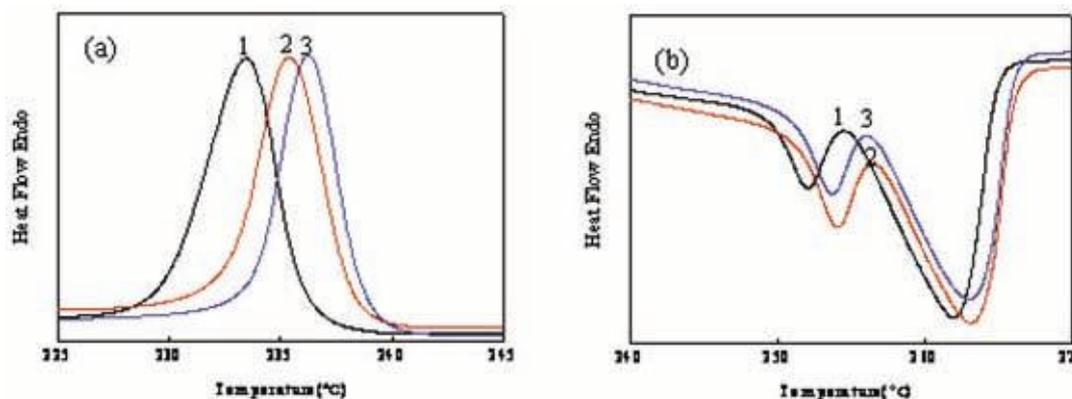
**Figure 4.** (a) DSC crystallization exotherms of PA66 and its nanocomposites and (b) DSC melting endotherms during the second heating cycle of PA 66 and its nanocomposites.
