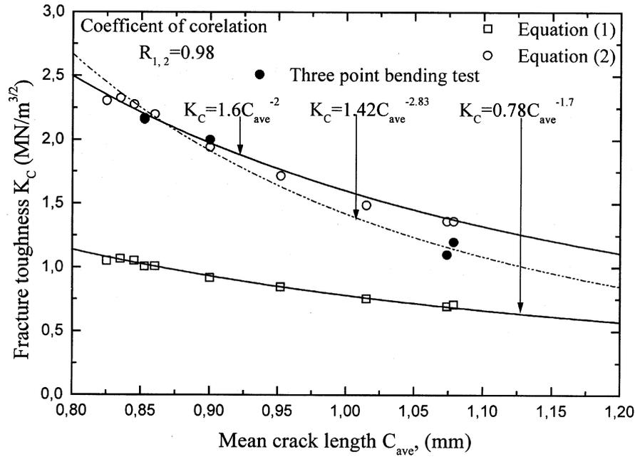
Figure 5. Theoretical and experimental fracture toughness of studied material vs mean crack length.
