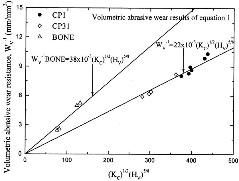
Figure 6. Abrasive wear resistance of bio-active glass ceramics and cortical bone according to  $K_c$  obtained from (1).
