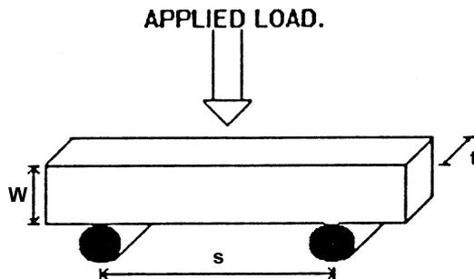
Figure 4. Schematic diagram of the three-point bending test.
