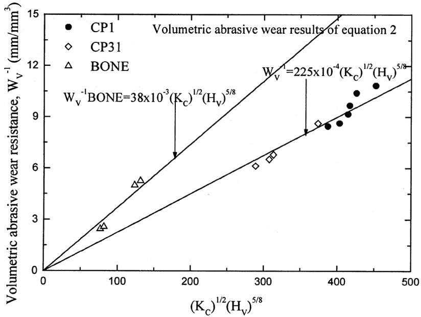
Figure 7. Abrasive wear resistance of bio-active glass ceramics and cortical bone according to  $K_c$  obtained from (2).
