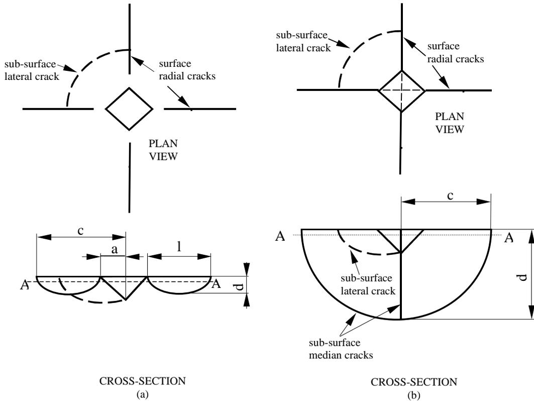
**Figure 2.** (a) Schematic plan and cross-sectional views of an idealized Vickers indent Palmqvist crack system and (b) schematic plan and cross-sectional views of an idealized Vickers indent radial-medial or half penny crack system.
