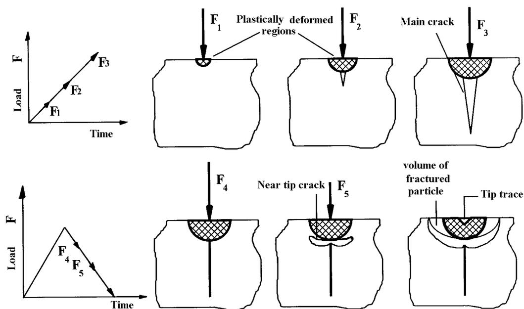
**Figure 1.** Main crack and near tip cracks after indentation of a sharp rigid tip.**Table 2.** Constituents of studied bio-active glass ceramics.
