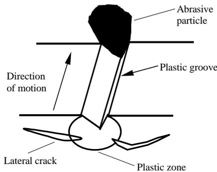
**Figure 3.** Schematic illustration of material removal in a brittle material by extension of lateral cracks from beneath a plastic groove (Srawley 1976; Ponton and Rawlings 1989; Alanyali 1992).
