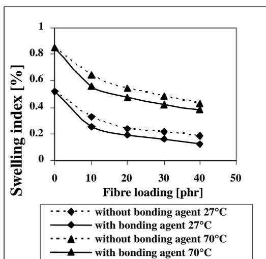
Figure 5. Variation of the % swelling index with fibre loading for the composites cured at 100°C in lubricating oil at 27°C and 70°C.
