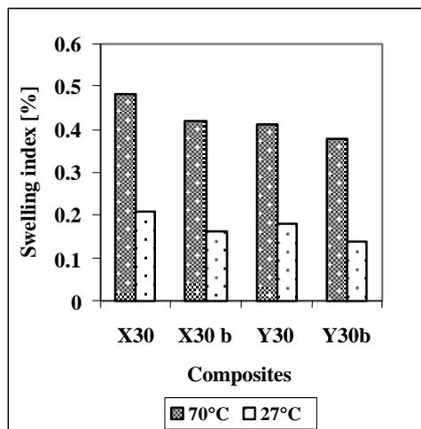
Figure 6. A comparison of the % swelling index for the composite (30 phr) containing untreated and alkali treated fibres in lubricating oil at 27°C and 70°C.
