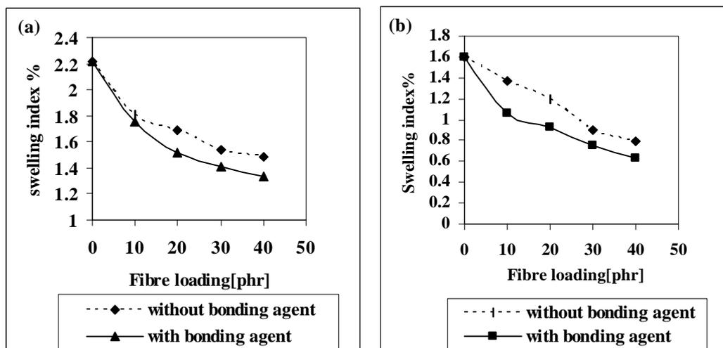
**Figure 4.** Variation of the % swelling index with fibre loading for the composites cured at 100°C in (a) petrol and (b) diesel.
