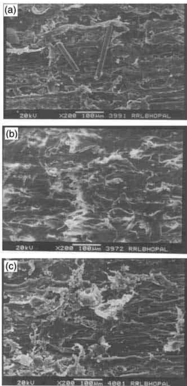
**Figure 5.** SEM micrographs of worn surfaces of LL-GF/LCP samples: (a) 90-75/25, (b) 90-50/50 and (c) 90-25/75 abraded at 7N load.
