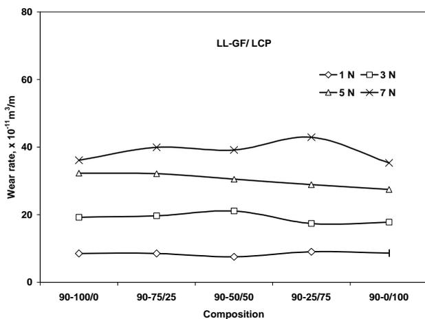
Figure 3. Plots between wear rate and composition for hybrid fibre composites having 10 vol.% fibres at different applied loads.
