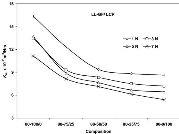
**Figure 7.** Plots between specific wear rate and composition of fibres in a composite having 20 vol.% fibres.
