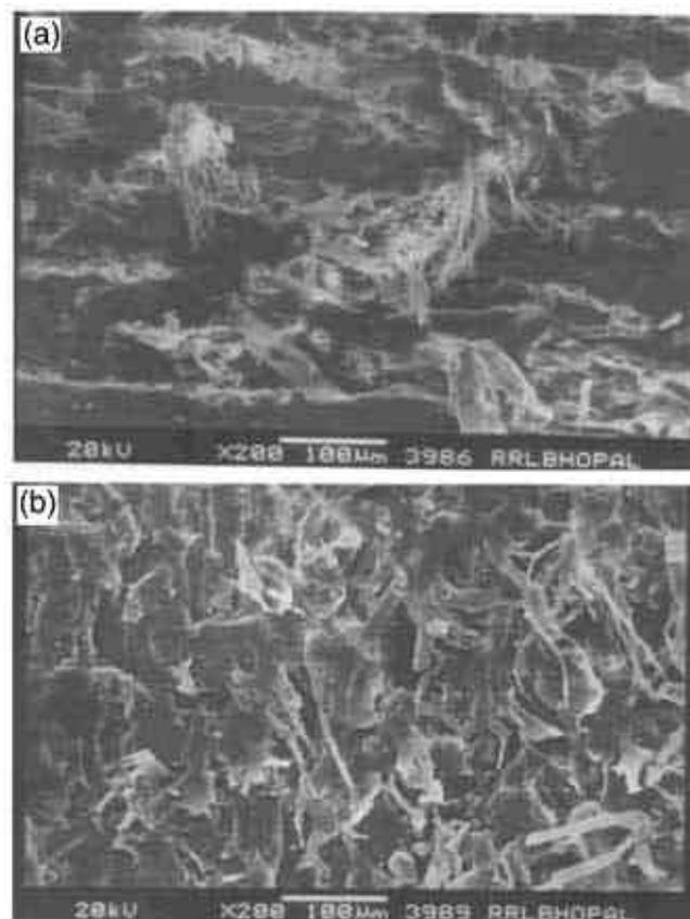
**Figure 6.** SEM micrographs of worn surfaces of LL-GF/LCP samples: (a) 80-50/50 and (b) 80-25/75 abraded at 7N load.
