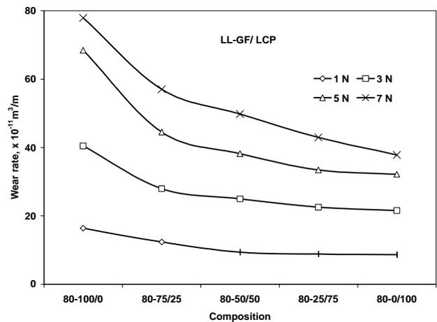
Figure 4. Plots between wear rate and composition for LLDPE and hybrid fibre composites having 20 vol.% fibres at different applied loads.
