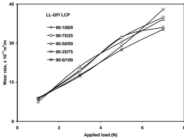
Figure 2. Plots between wear rate and applied load for different composites having 10 vol.% fibres in LLDPE.
