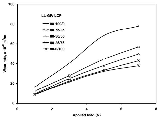
**Figure 1.** Plots between wear rate and applied load for different composites having 20 vol.% fibres in LLDPE.
