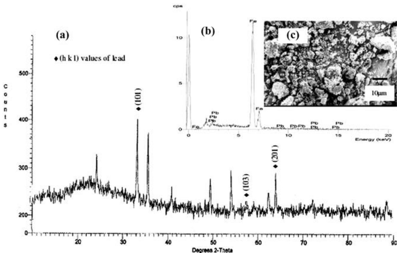
**Figure 2.** (a) XRD pattern of lead adsorbed  $\alpha$ -Fe<sub>2</sub>O<sub>3</sub>, (b) EDX spectra of lead adsorbed  $\alpha$ -Fe<sub>2</sub>O<sub>3</sub> and (c) SEM image of lead adsorbed  $\alpha$ -Fe<sub>2</sub>O<sub>3</sub>.
