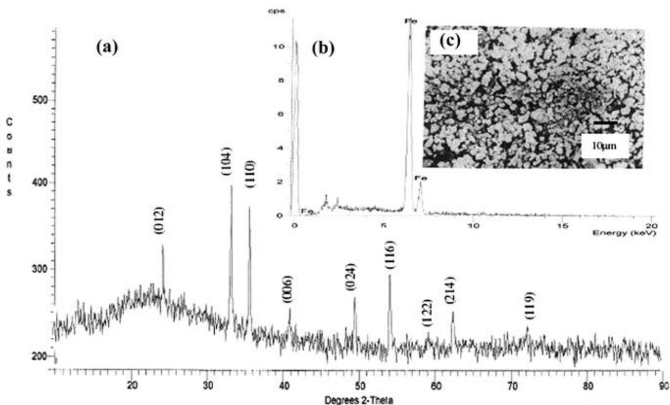
**Figure 1.** (a) XRD pattern of  $\alpha$ -Fe<sub>2</sub>O<sub>3</sub>, (b) EDX spectra of  $\alpha$ -Fe<sub>2</sub>O<sub>3</sub> and (c) SEM image of  $\alpha$ -Fe<sub>2</sub>O<sub>3</sub>.
