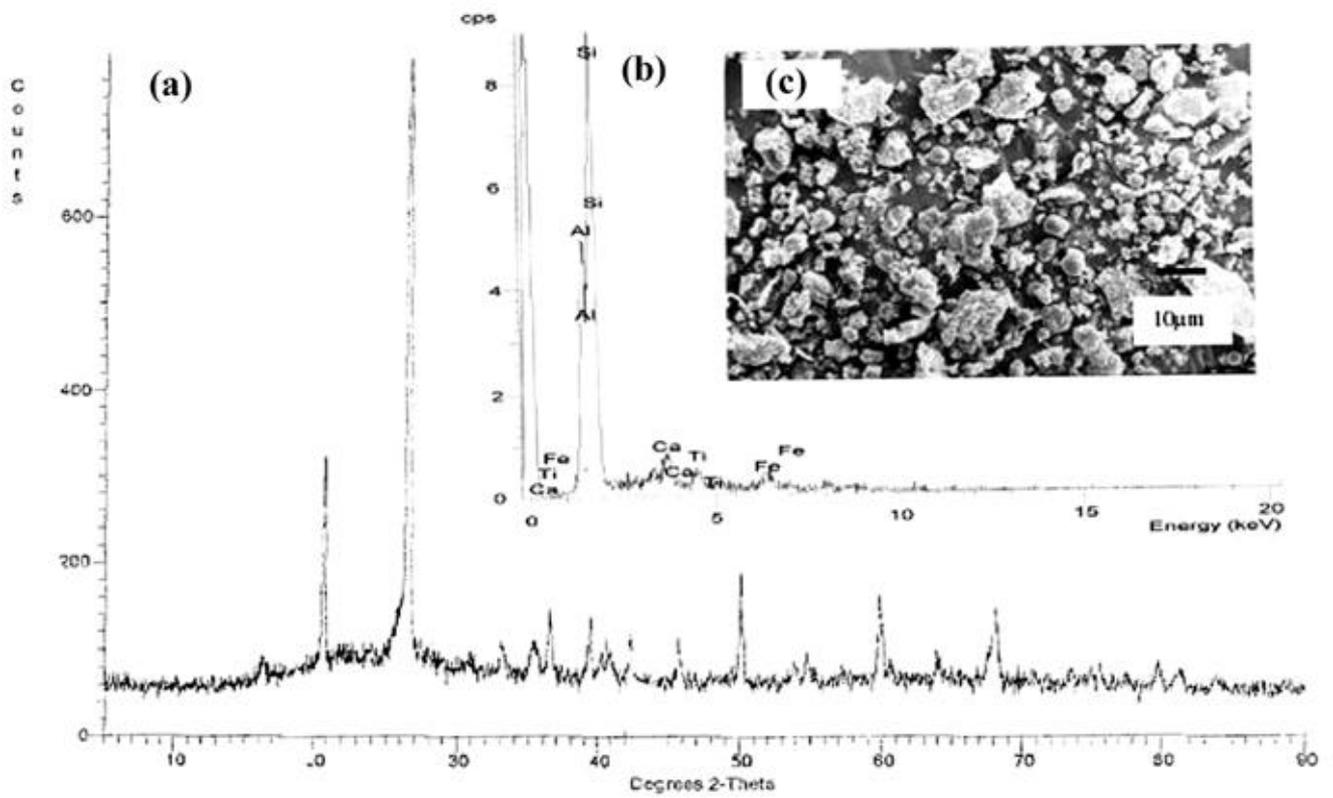
Figure 3. (a) XRD pattern of fly ash, (b) EDX spectra of fly ash and (c) SEM image of fly ash.
