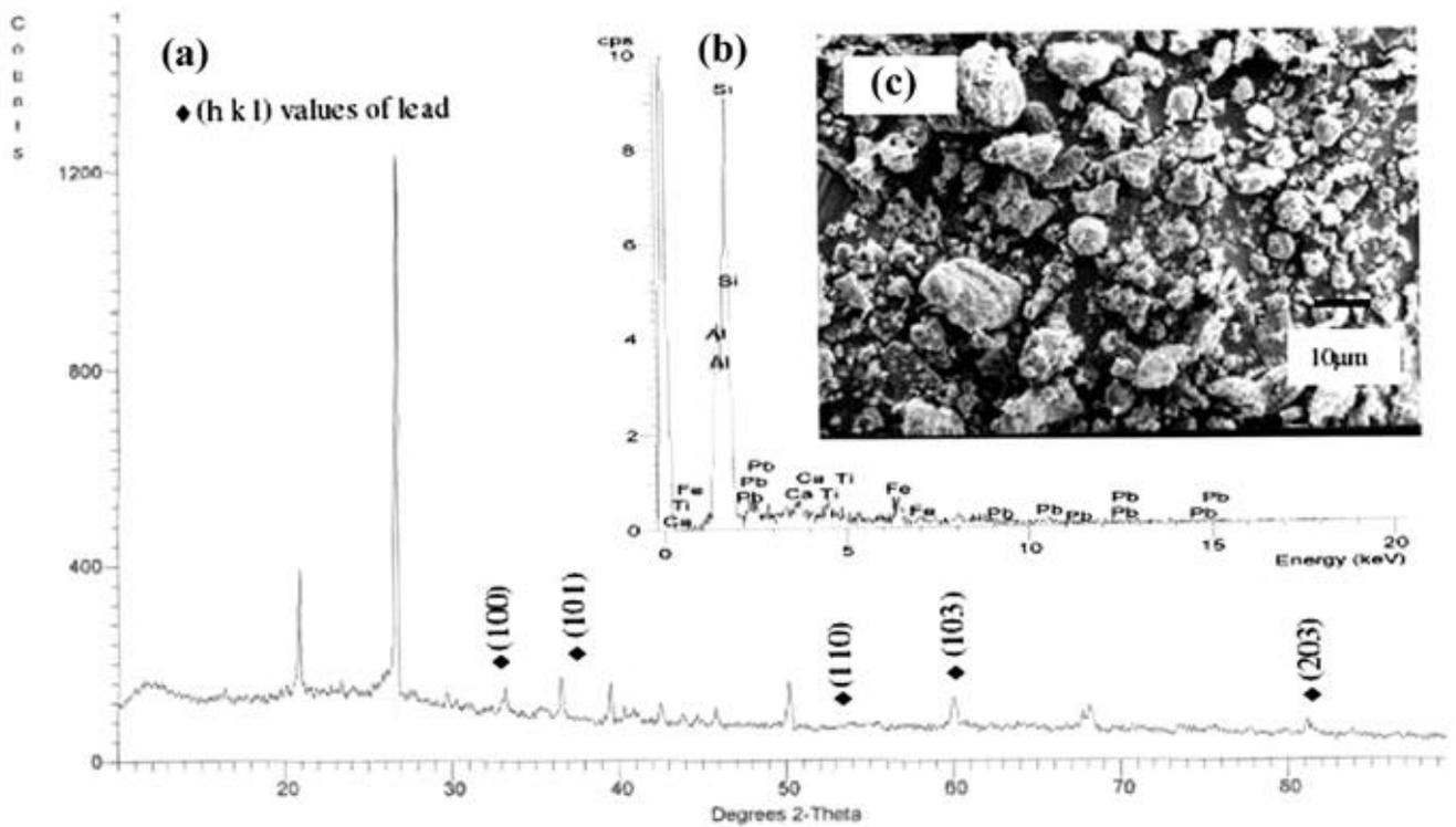
Figure 4. (a) XRD pattern of lead adsorbed fly ash, (b) EDX of lead adsorbed fly ash and (c) SEM image of lead adsorbed fly ash.
