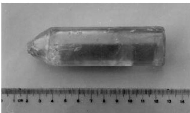
Figure 6.  $\text{PbMoO}_4$  crystal grown by modified Bridgman method.
