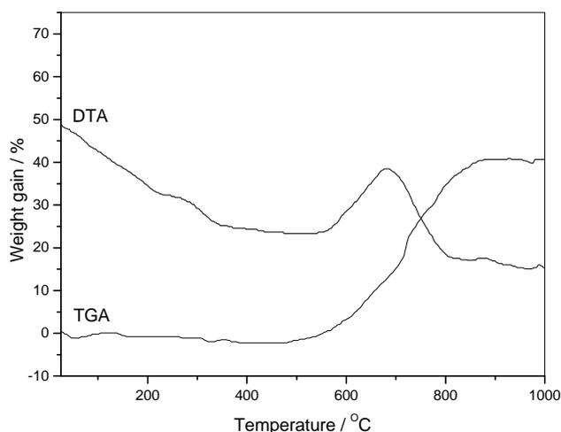
Figure 3. TGA/DTA curves of  $\text{WSi}_2$  heated in flowing air.
