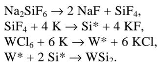
In this route, NaF, KF and KCl can be formed as by-products. The melting point of the salt system is about 605–606°C. Since the reaction temperature is above this melting point, the reaction, in which nascent tungsten (W\*) combines with nascent silicon (Si\*) to form tungsten disilicide, can be carried out in this molten salt system. The molten salt helps to form the nanocrystalline tungsten disilicide.
