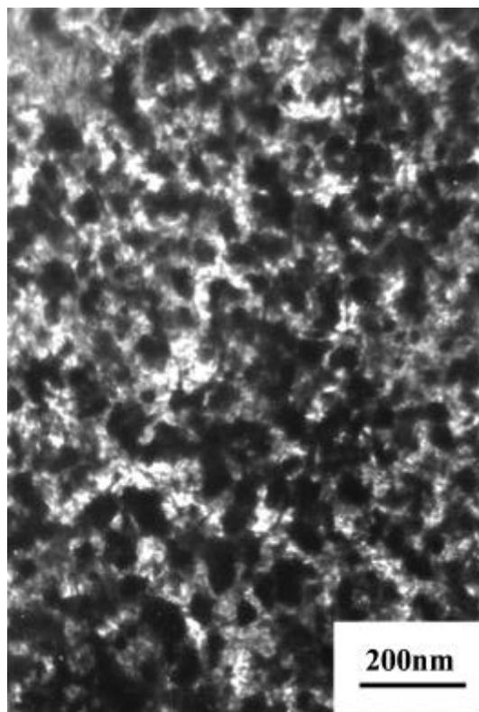
Figure 2. TEM image of the as-prepared  $\text{WSi}_2$  sample.
