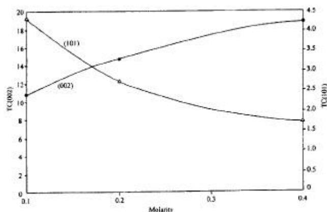
**Figure 4.** Variation of texture coefficient  $TC(002)$  and  $TC(101)$  of 0.8 at.% zinc oxide films deposited at  $723 \pm 5$  K using zinc acetate solution of different molarities.
