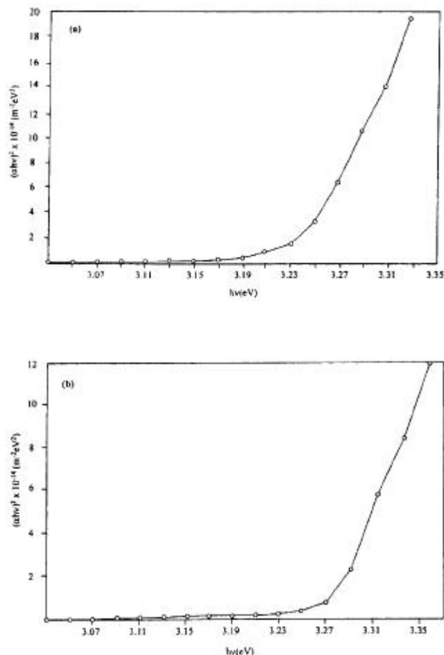
**Figure 7.** Typical variation of  $(ahv)^2$  vs  $h\nu$  of zinc oxide films deposited at  $723 \pm 5$  K using 0.1 M zinc acetate solution with different indium doping concentrations (a) 0 and (b) 0.8 at.%.
