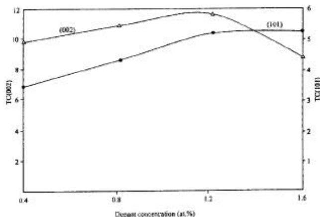
**Figure 2.** Variation of texture coefficient  $TC(002)$  and  $TC(101)$  of zinc oxide films deposited at  $723 \pm 5$  K using 0.1 M zinc acetate solution with different indium concentrations.
