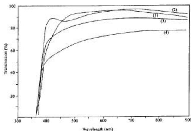
**Figure 6.** Optical transmission spectra of indium doped zinc oxide films deposited at a substrate temperature of  $723 \pm 5$  K using 0.1 M zinc acetate solution for different indium concentrations: (1) 0, (2) 0.4 at%, (3) 1.2 at% and (4) 1.6 at%.
