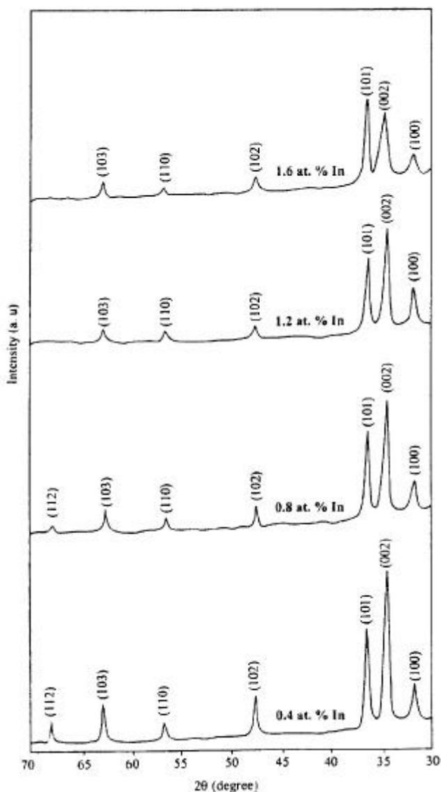
**Figure 1.** XRD patterns of IZO films deposited at  $723 \pm 5$  K using 0.1 M zinc acetate solution with different indium concentrations.
