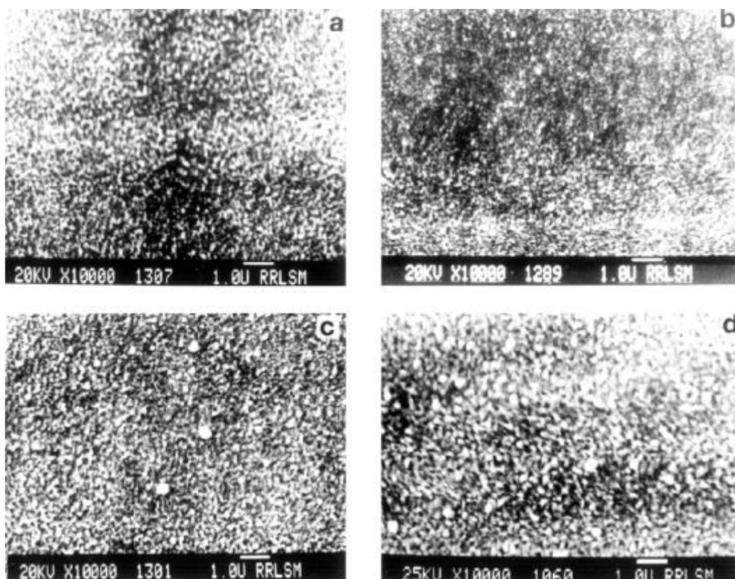
**Figure 5.** SEM photographs of IZO films deposited at  $723 \pm 5$  K using 0.1 M zinc acetate solution with different indium concentrations: **a.** 0, **b.** 0.4 at.%, **c.** 1.2 at.% and **d.** 1.6 at.%.
