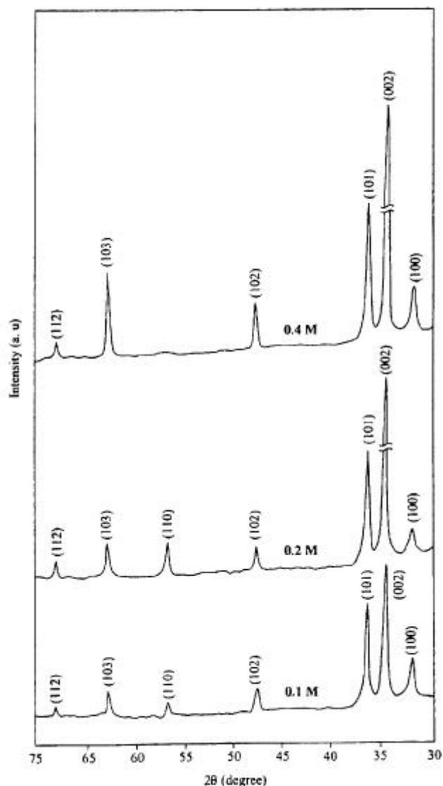
**Figure 3.** XRD patterns of 0.8 at.% indium doped zinc oxide films prepared at  $723 \pm 5$  K using zinc acetate solutions of different molarities.
