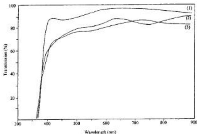
**Figure 8.** Optical transmission spectra of 0.8 at.% indium doped zinc oxide films deposited at a substrate temperature of  $723 \pm 5$  K using zinc acetate solutions of different molarities: (1) 0.1, (2) 0.2 and (3) 0.4 M.
