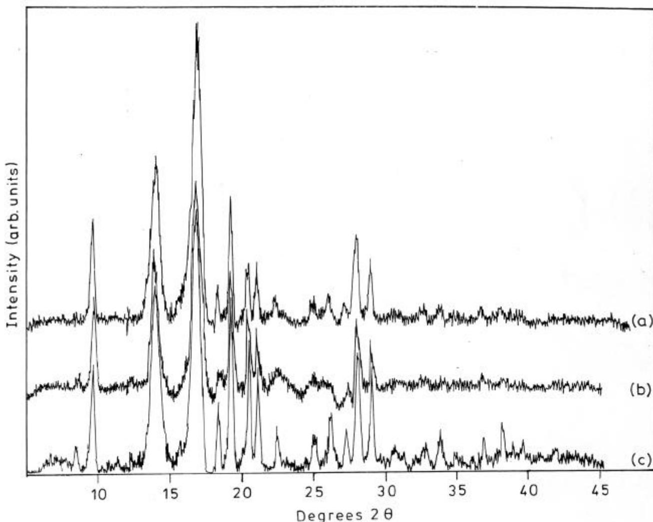
Figure 1. Powder X-ray diffraction pattern of (a) 20% CTC, (b) 60% CTC and (c) pure CTC.
