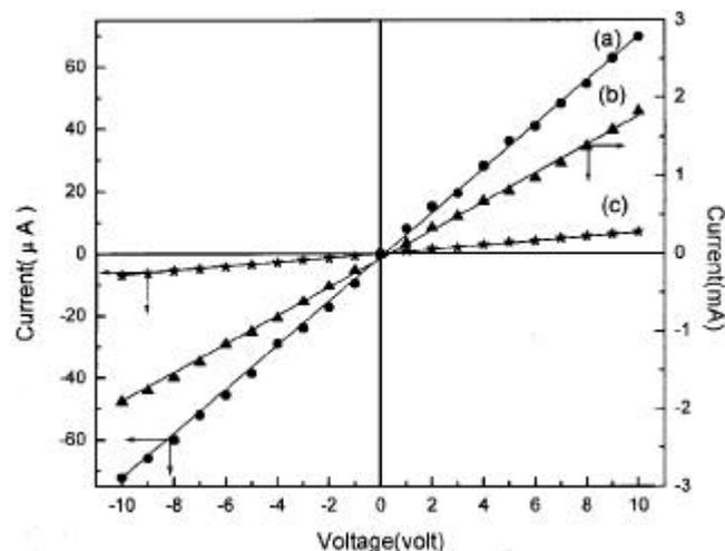
**Figure 2.** Current-voltage characteristics of phenothiazine-iodine-PS (a) 60% CTC, (b) pure CTC and (c) 20% CTC.
