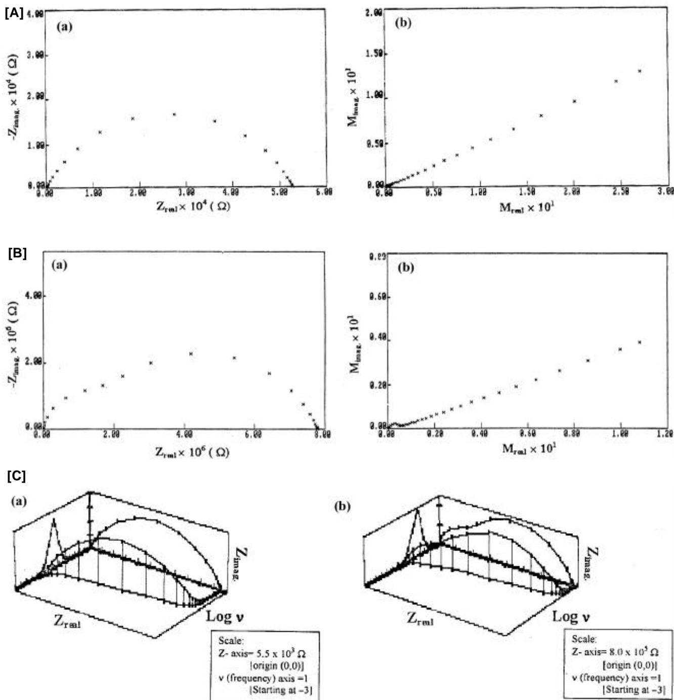
**Figure 6.** A. Complex impedance plots for phenothiazine-iodine-PS for 60 wt% CTC composite: (a) complex impedance plot and (b) complex modulus plot, B. complex impedance plots for phenothiazine-iodine-PS for 20 wt% CTC composite: (a) complex impedance plot and (b) complex modulus plot and C. three-dimensional perspective plots for phenothiazine-iodine-PS: (a) 60 wt% CTC and (b) 20 wt% CTC.
