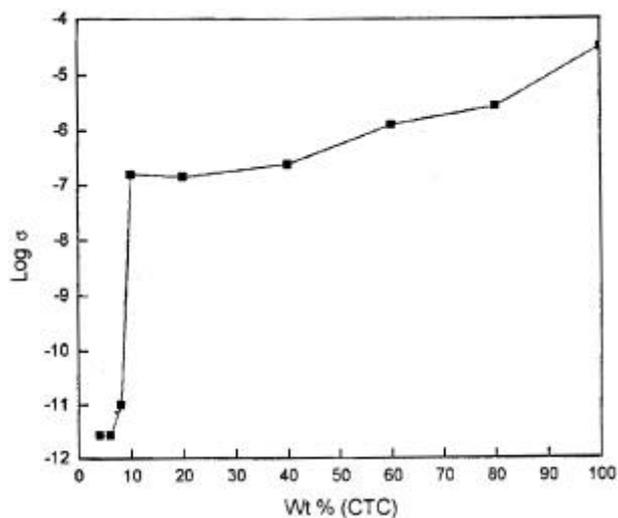
**Figure 4.** Variation of specific conductance of composite as a function of amount of charge-transfer complex.
