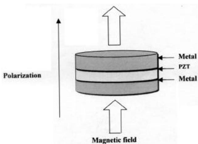
Figure 1. The schematic structure of a laminate composite.
