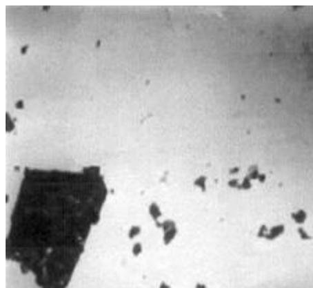
Figure 4. Optical micrograph of  $Zn_{1-x}Mn_xTe$  for  $x = 0.50$  at  $100\times$ .
