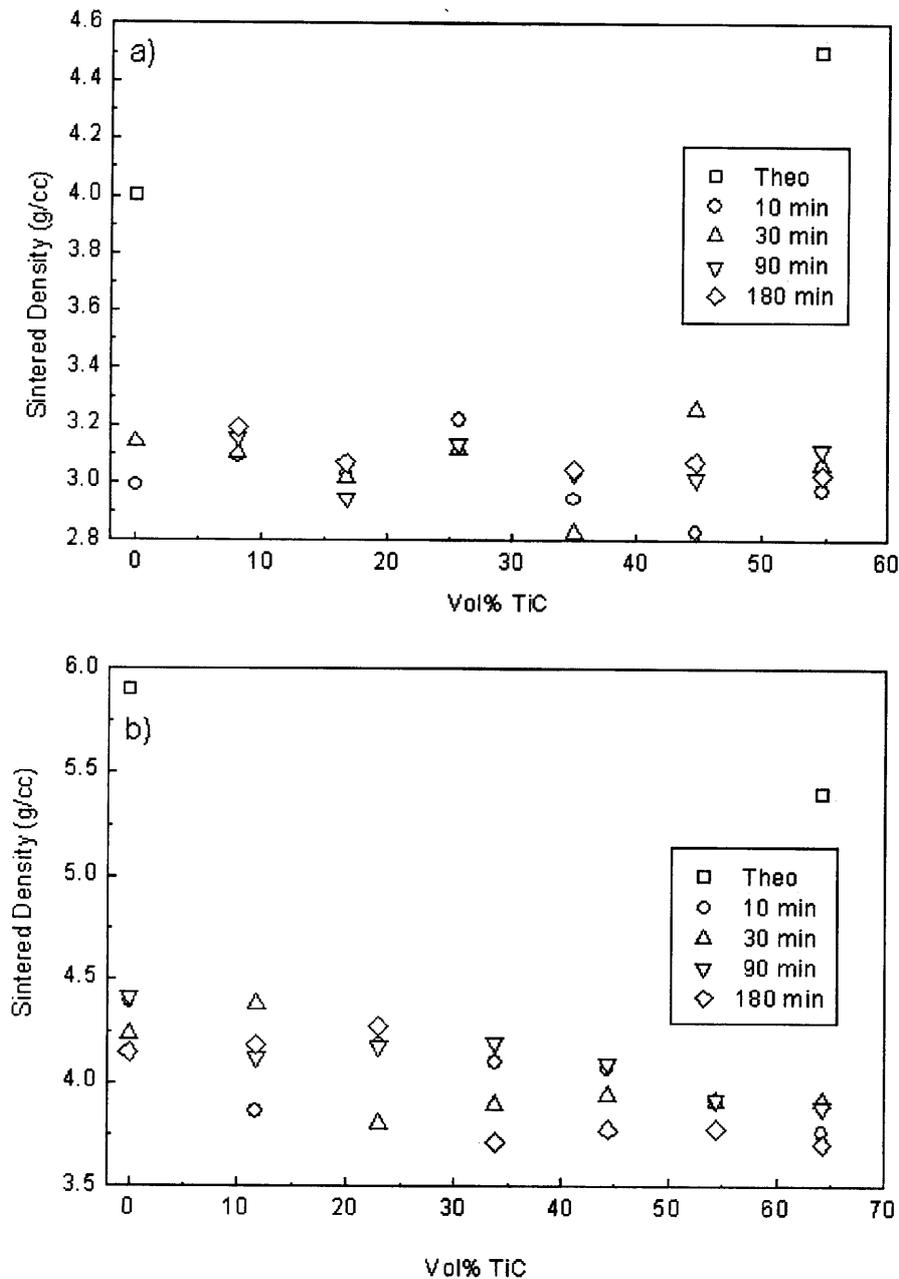
**Figure 1.** Variation of sintered density of (a) Al<sub>2</sub>O<sub>3</sub>-TiC and (b) ZrO<sub>2</sub>-TiC with amount of TiC sintered at 1600°C at different soaking times.
