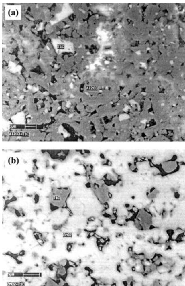
**Figure 2.** SEM micrograph of (a) 74.3 Al<sub>2</sub>O<sub>3</sub>-25.7 vol.% TiC composite and (b) 66.25 ZrO<sub>2</sub>-33.75 vol.% TiC composite.
