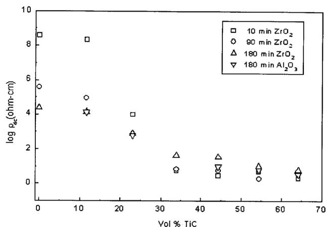
**Figure 3.** Variation of d.c. resistivity of Al<sub>2</sub>O<sub>3</sub> and ZrO<sub>2</sub> composites with TiC.
