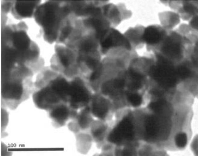
Figure 2. TEM of BN powder calcined at 600°C.
