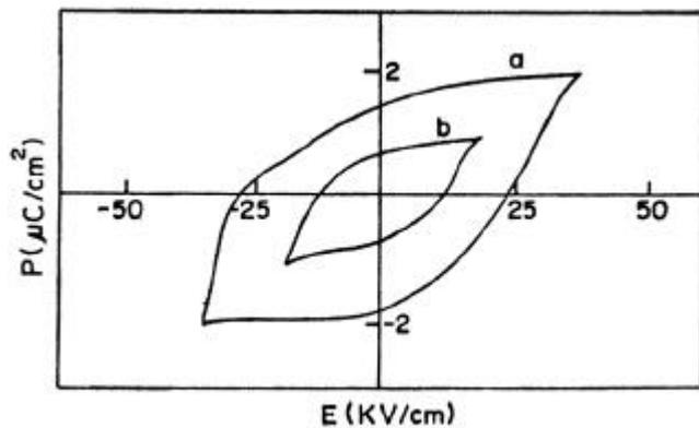
Figure 3. P/E loop measurements for (a) citrate derived and (b) solid state method derived samples.
