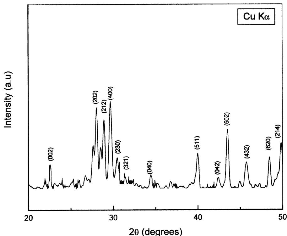
Figure 1. XRD of BN powder calcined at  $600^\circ\text{C}$ .
