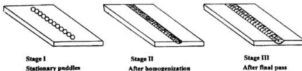
**Figure 1.** Various stages of weld simulation by elemental implant technique.
