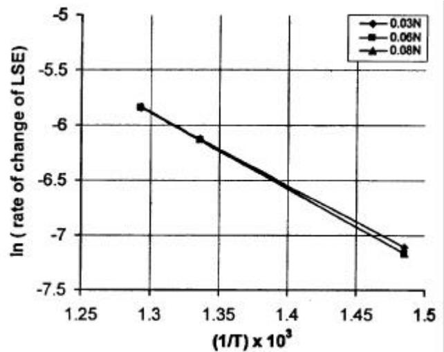
Figure 5. Arrhenius plot for the calculation of activation energy.
