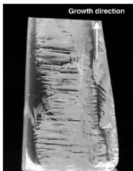
**Figure 3.** Featherlike striations in as-grown  $\text{Nd}^{3+}:\text{SGG}$  crystal.
