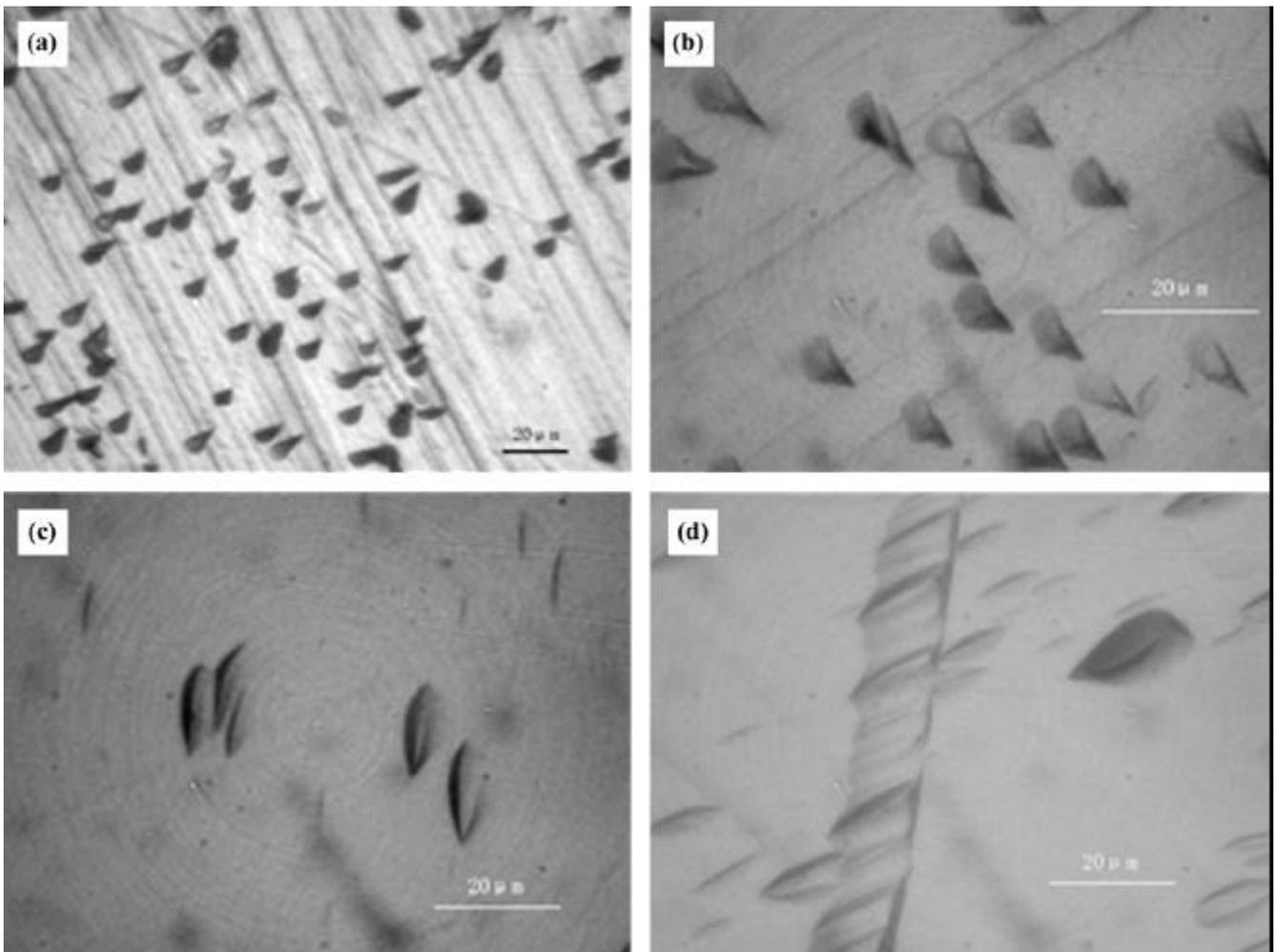
**Figure 5.** The etch pits of  $\text{Nd}^{3+} : \text{SGG}$  crystal. The etch pits distribution on (a) (001) plane, (b) (201) plane, (c) (111) plane and (d) (111) plane of  $\text{Nd}^{3+} : \text{SGG}$  crystals.
