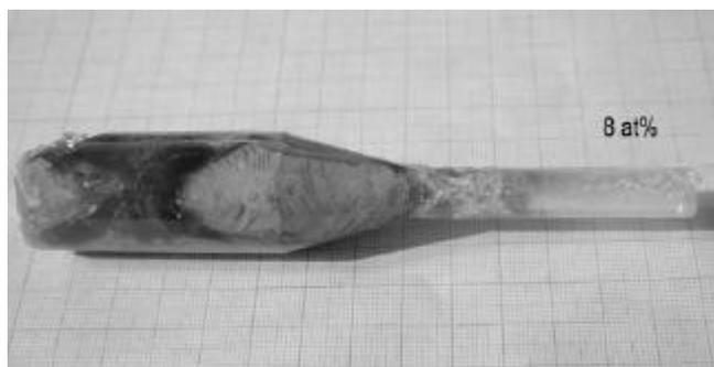
**Figure 2.** As-grown SGG crystals doped with 8 at%  $\text{Nd}^{3+}$  ions covered with impurities.
