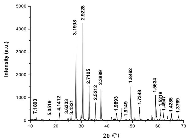
**Figure 1.** Powder X-ray diffraction pattern of SGG polycrystalline obtained by solid-state reaction.
