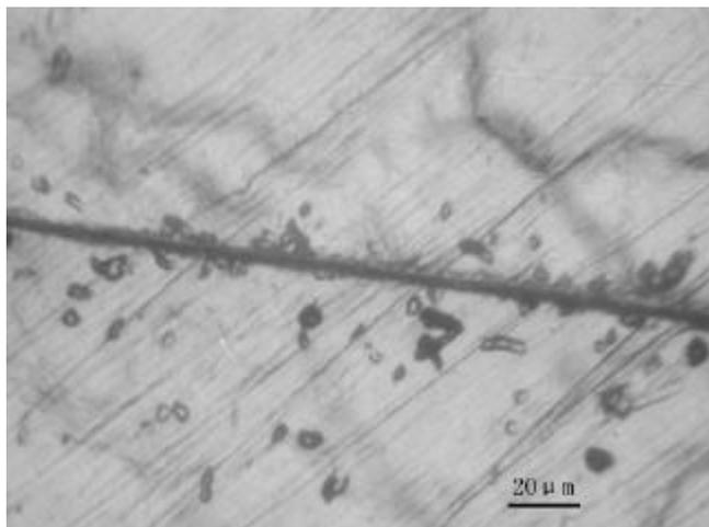
**Figure 6.** The distribution of etch pits near the micro-crack.
