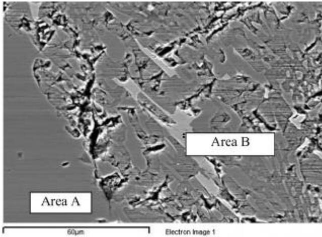
**Figure 4.** Morphology of the inclusions in  $\text{Nd}^{3+} : \text{SGG}$  crystal.
