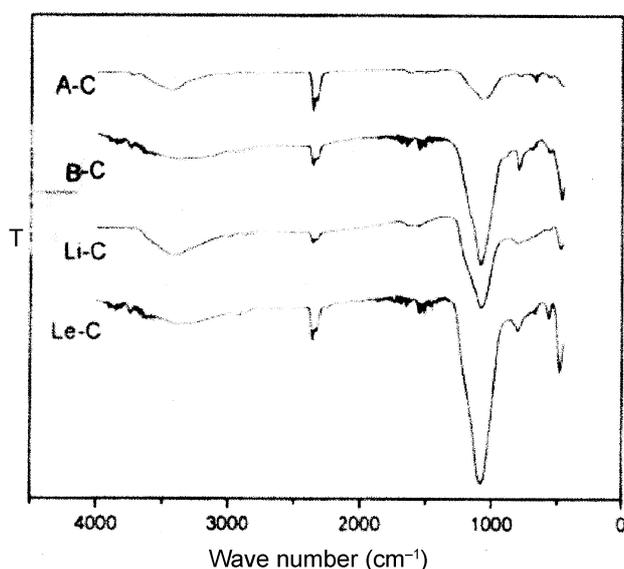
Figure 10. FT-IR spectra of the carbonized products.
