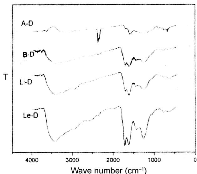
Figure 15. FT-IR spectra of the demineralized products.
