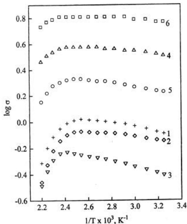
**Figure 3.** Conductivity of Pani materials as a function of temperature: (1) Pani-SO<sub>4</sub><sup>2-</sup>, (2) Pani-SO<sub>4</sub><sup>2-</sup>/TOCr, (3) Pani-SO<sub>4</sub><sup>2-</sup>/TOFe, (4) Pani-SO<sub>4</sub><sup>2-</sup>/TOMn, (5) Pani-SO<sub>4</sub><sup>2-</sup>/TOCo and (6) Pani-SO<sub>4</sub><sup>2-</sup>/TOAl.
