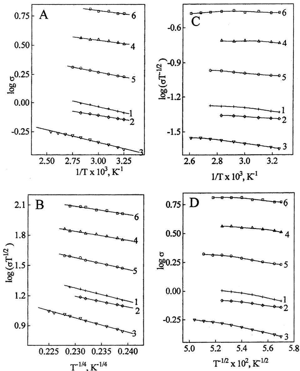
**Figure 4.** A. Arrhenius plot and (B, C and D) plots of VRH, GB and TC mechanisms of (1) Pani-SO<sub>4</sub><sup>2-</sup>, (2) Pani-SO<sub>4</sub><sup>2-</sup>/TOCr, (3) Pani-SO<sub>4</sub><sup>2-</sup>/TOFe, (4) Pani-SO<sub>4</sub><sup>2-</sup>/TOMn, (5) Pani-SO<sub>4</sub><sup>2-</sup>/TOCo and (6) Pani-SO<sub>4</sub><sup>2-</sup>/TOAl. (Plots were drawn using Origin 4.0 software. A and B – linear-fit plots; C and D polynomial plots with order 4 or 5).
