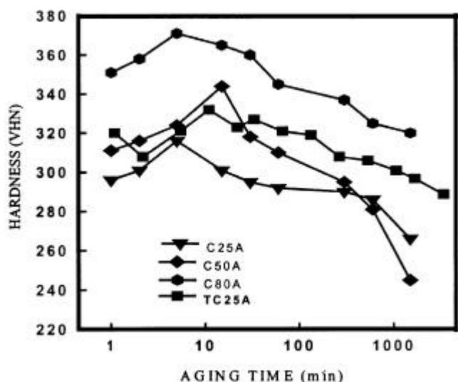
Figure 1. Variation of hardness with aging time.
