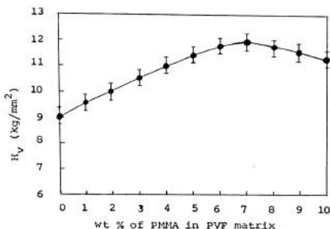
**Figure 1.** Variation of  $H_v$  with different wt% of PMMA in PVF : PMMA polyblend specimens at the saturation load of 80 g.
