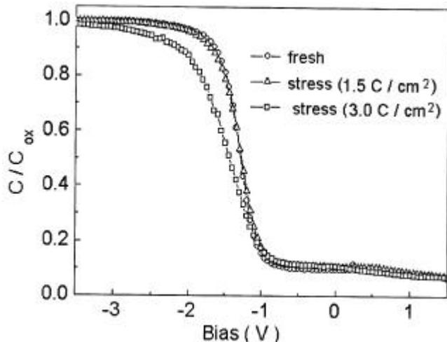
**Figure 6.** High frequency (1 MHz)  $C$ - $V$  characteristics of MIS structures: before and after stressing.
