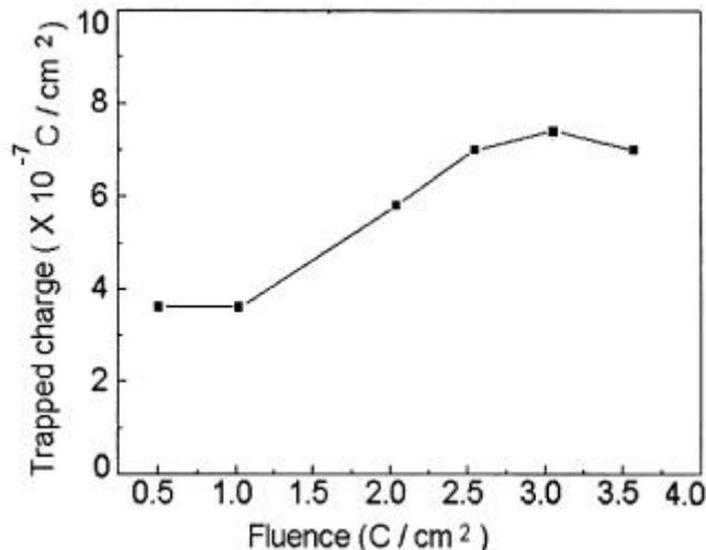
**Figure 8.** The density of trapped charges vs fluence under constant current injection.
