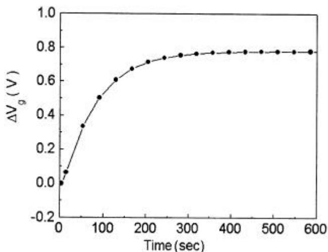
**Figure 7.** Gate voltage shift vs stress time under constant current stressing ( $-5 \text{ mA/cm}^2$ ).
