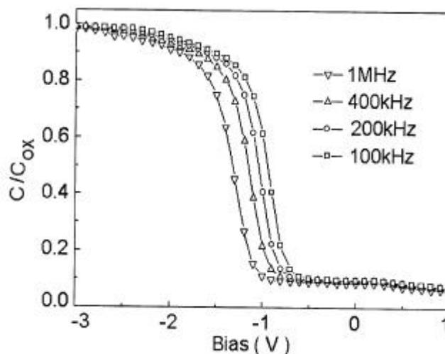
**Figure 5.**  $C$ – $V$  characteristics at different frequencies for Ta<sub>2</sub>O<sub>5</sub>/ZnO/ $p$ -Si MIS structures.
