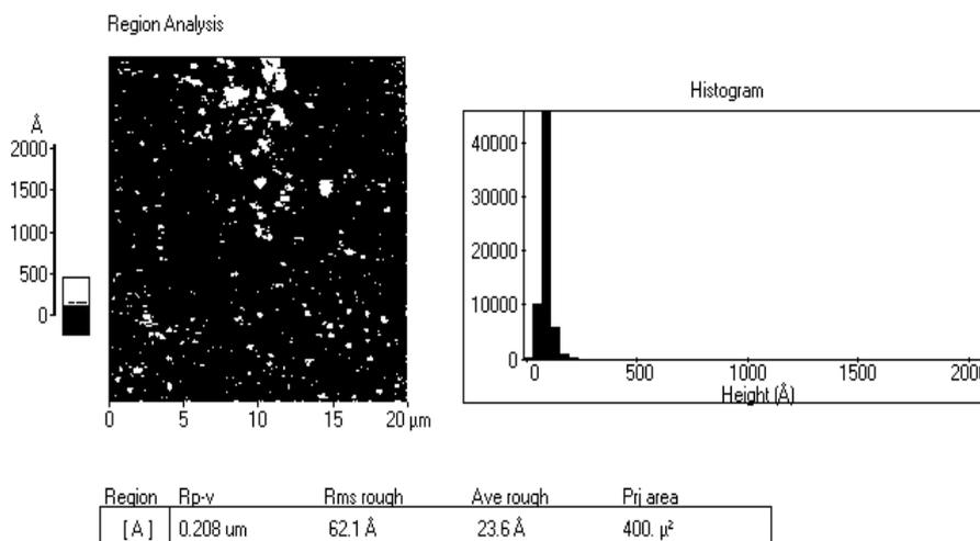
Figure 2. Two-dimensional AFM image of the ZnO film.
