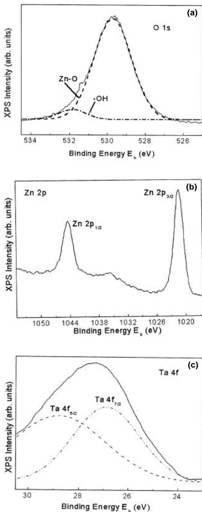
**Figure 4.** X-ray photoelectron spectroscopy results of the (a) O 1s, (b) Zn 2p and (c) Ta 4f peaks of Ta<sub>2</sub>O<sub>5</sub>/ZnO/Si films.
