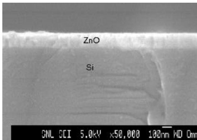
Figure 3. Cross-sectional SEM view of the rf sputtered ZnO film deposited on *p*-Si.
