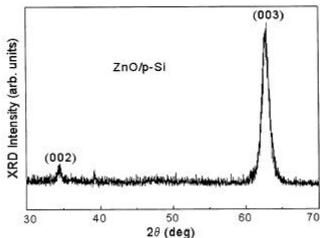
Figure 1. X-ray diffraction pattern of ZnO thin films.
