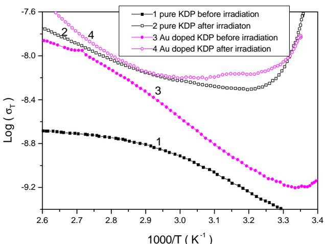
Figure 7. Variation of  $\log(\sigma_T)$  with  $1000/T$  in pure KDP and  $\text{Au}^+$  doped KDP crystals before and after irradiation.
