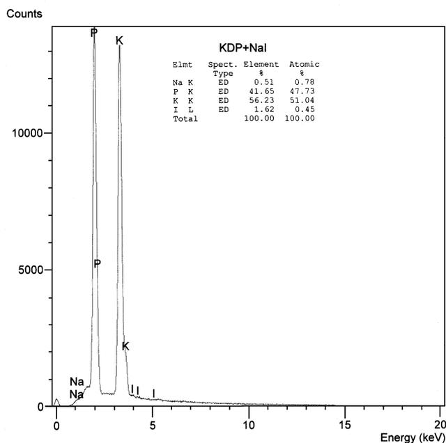
Figure 2. EDAX data of (KDP)<sub>0.8</sub> (NaI)<sub>0.2</sub> crystals.
