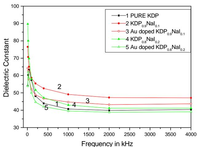
**Figure 4.** Variation of dielectric constant with frequency in KDP crystals containing NaI with and without gold doping.
