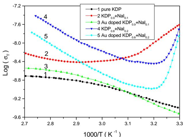
Figure 6. Variation of  $\log(\sigma_T)$  with  $1000/T$  in KDP crystals containing NaI with and without gold doping.
