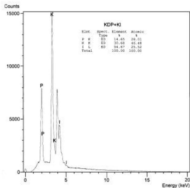
Figure 1. EDAX data of (KDP)<sub>0.8</sub> (KI)<sub>0.2</sub> crystals.
