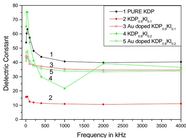
Figure 3. Variation of dielectric constant with frequency in KDP crystals containing KI with and without gold doping.
