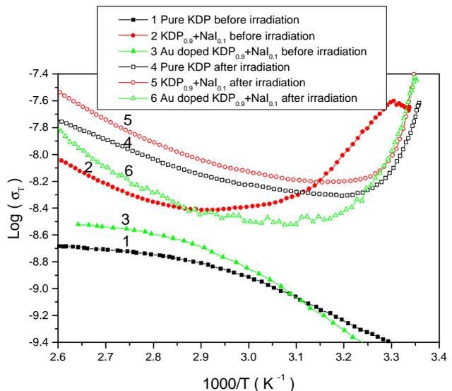
Figure 9. Variation of  $\log(\sigma_T)$  with  $1000/T$  in KDP crystals containing NaI with and without gold doping before and after irradiation.
