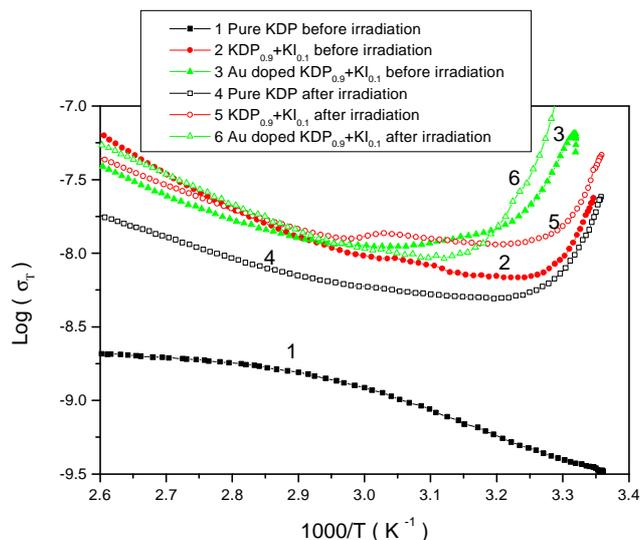
Figure 8. Variation of  $\log(\sigma_T)$  with  $1000/T$  in KDP crystals containing KI with and without gold doping before and after irradiation.
