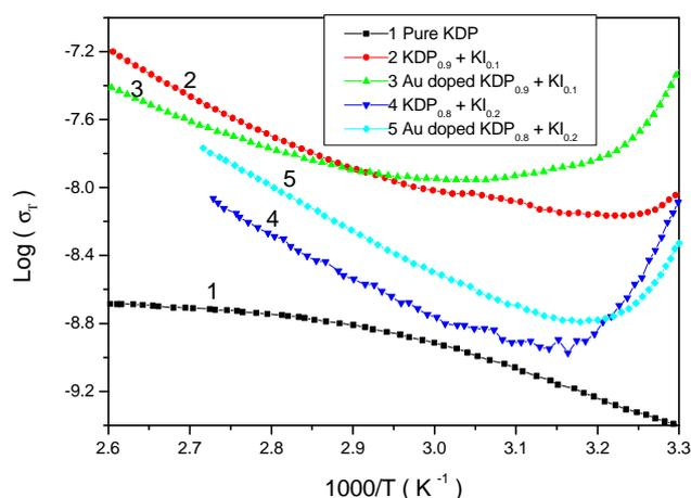
**Figure 5.** Variation of  $\log(s_T)$  with  $1000/T$  in KDP crystals containing KI with and without gold doping.
