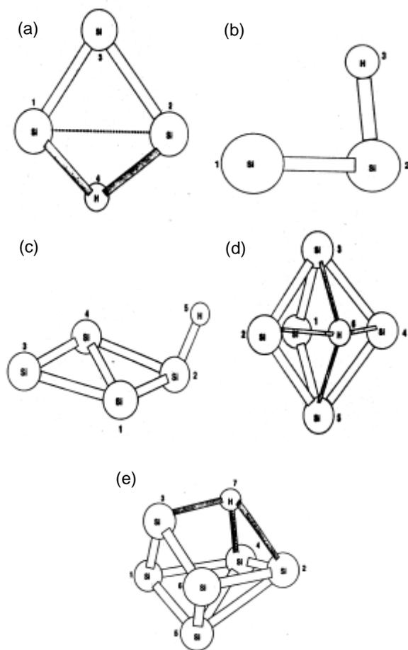
**Figure 1.** Ground state geometry of (a)  $\text{Si}_2\text{H}$ , (b)  $\text{Si}_3\text{H}$ , (c)  $\text{Si}_4\text{H}$ , (d)  $\text{Si}_5\text{H}$  cluster and (e)  $\text{Si}_6\text{H}$  cluster.
