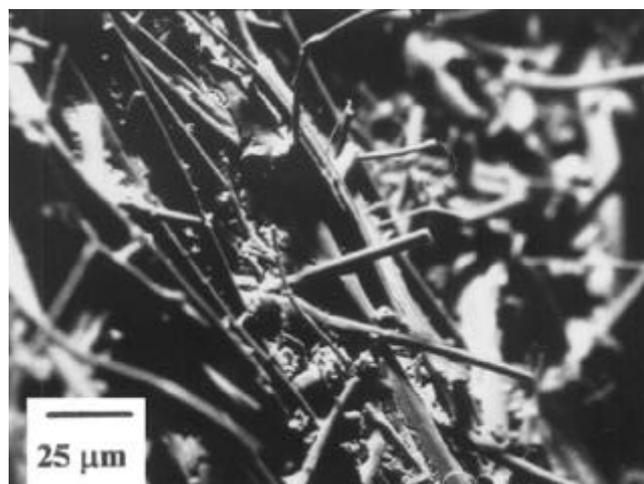
**Figure 3.** SEM of the fracture surface of the product of run no. 1 of table 1 showing fibre pull-out.
