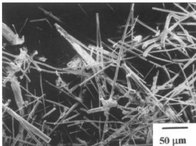
**Figure 2.** SEM of the as-received (uninfiltrated) mullite fibre preform.
