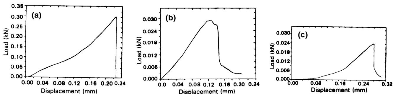
**Figure 1.** Load displacement curves of (a) the product of run no. 3 of table 1, (b) the product of run no. 1 of table 1 and (c) the ceramic specimen (without any fibre reinforcing material).
