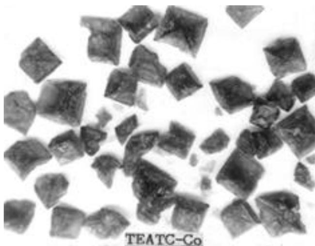
Figure 1. Photograph of the grown crystals of TEATC-Co.
