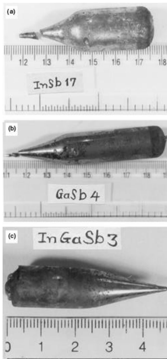
Figure 1. Typical as grown ingots: a. InSb17, b. GaSb-4 and c. InGaSb-3 represent the smooth and glossy surface without surface defects, indicating orientation growth due to self-seeding.
