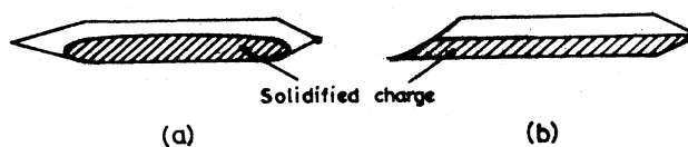
Figure 12. Ampoule shapes used in horizontal Bridgman experiments.
