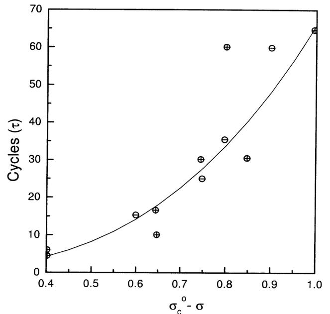
**Figure 2.** Plots of time-to-fracture  $t$  vs load  $s$  for different glasses:  $\oplus$  for sodalime,  $\otimes$  for borosilicate. The solid curve corresponds to (5) with  $1/\nu = 3$  and  $s_c^0 \approx 1.0$  N.
