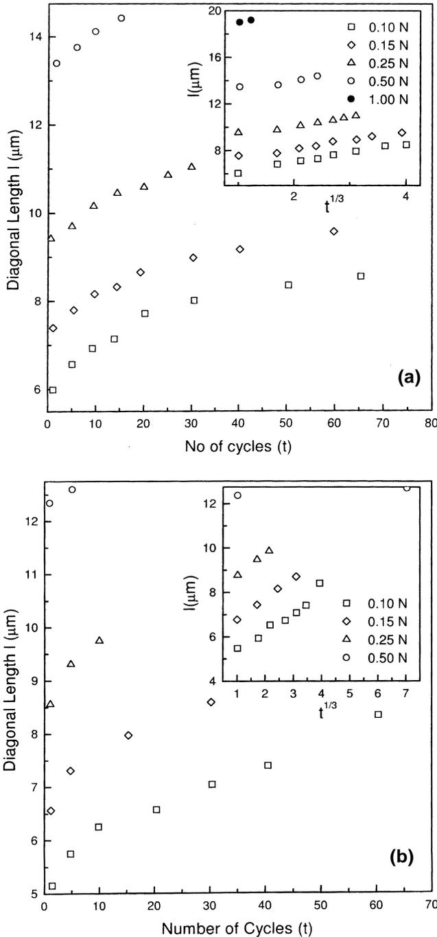
**Figure 1.** Plots of  $l(t)$  vs  $t$  for different  $s < s_c^0$ . Various symbols indicate different values of the external load:  $\square$  for 0.10 N,  $\diamond$  for 0.15 N,  $\Delta$  for 0.25 N,  $\circ$  for 0.50 N and  $\bullet$  for 1.0 N. The last data point in any set indicate the corresponding fracture point. The insets show the corresponding plots of  $l$  vs  $t^{1/3}$  (a) for sodalime and (b) for borosilicate glasses.
