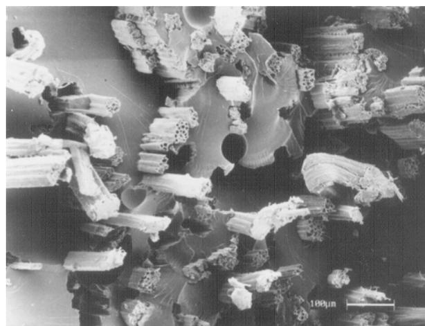
**Figure 11.** Transverse fracture of composites reinforced with 23 wt% 8 h alkali treated jute fibres.
