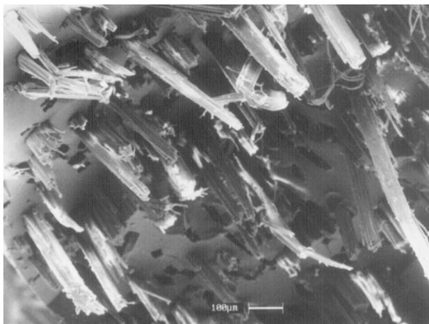
**Figure 9.** Fibre pull out and breakage in composites reinforced with 23 wt% untreated jute fibres.
