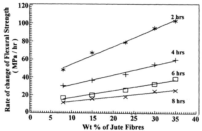
Figure 4. Variation of the rate of change of flexural strength of composites with varying wt% of alkali treated jute fibres.
