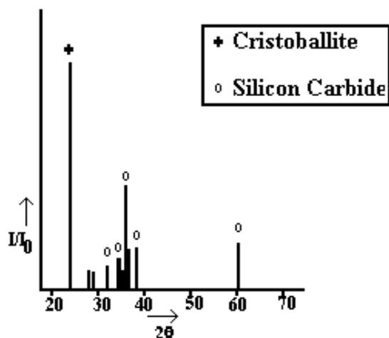
**Figure 6.** XRD lines of conventionally fired silicon carbide.
