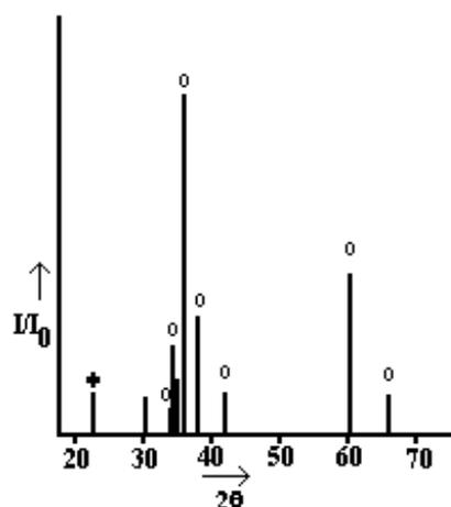
**Figure 5.** XRD lines of microwave fired silicon carbide.
