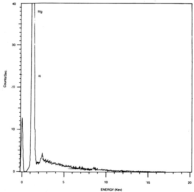
Figure 12. EDX pattern of the bulk matrix.
