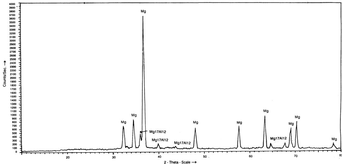
**Figure 7.** X-ray diffraction pattern of the sample without Pb.
