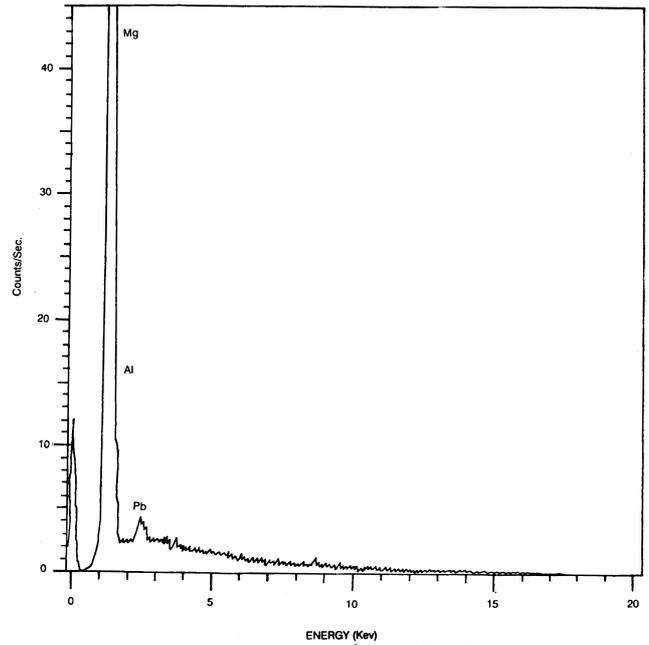
Figure 11. EDX pattern of the depleted matrix in the DP nodule.
