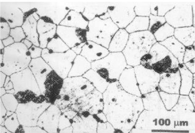
**Figure 4.** Microstructure of the Mg–Al alloy without Pb showing DP nodules (aged at 523 K for 4 h).
