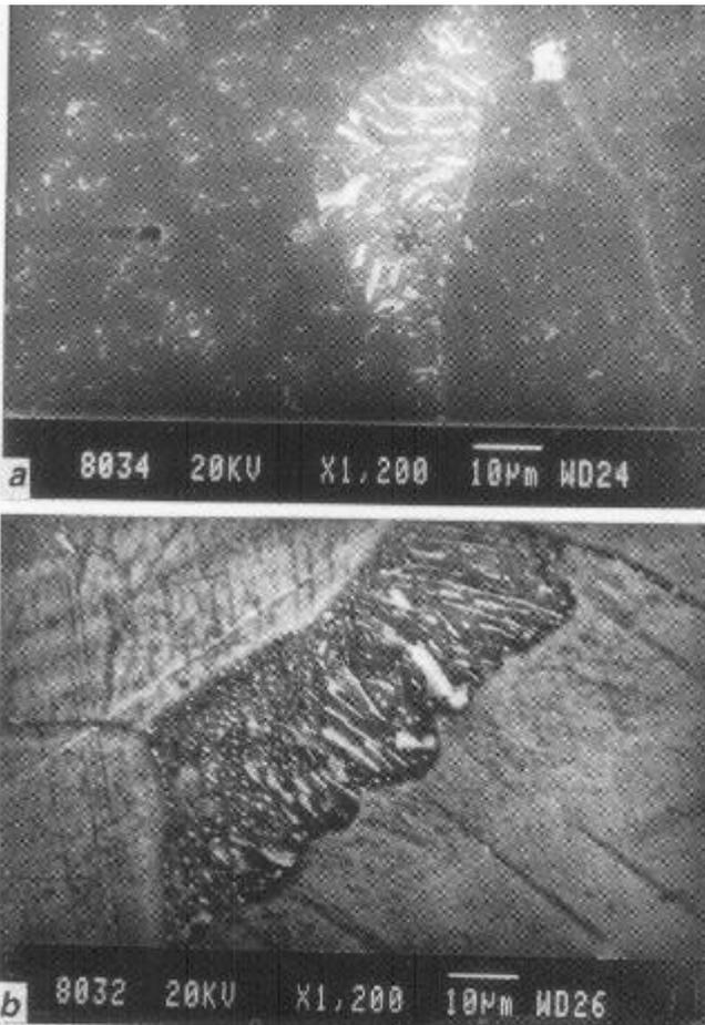
Figure 9. SEM of DP nodule for Mg–Al alloy without Pb (a) and with Pb (b).
