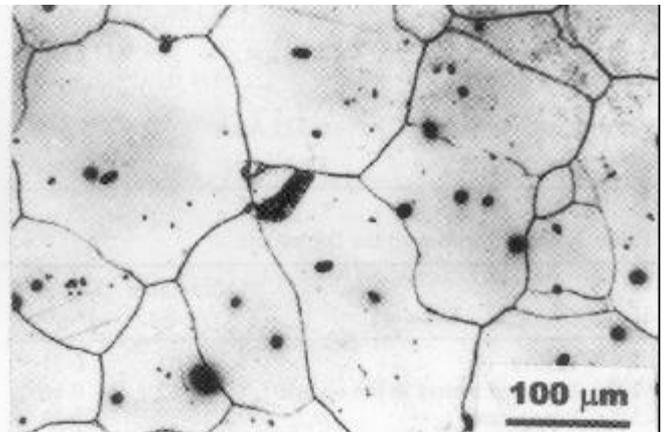
**Figure 5.** Microstructure of the Mg–Al alloy with Pb showing insignificant DP nodules (aged at 523 K for 2 h).
