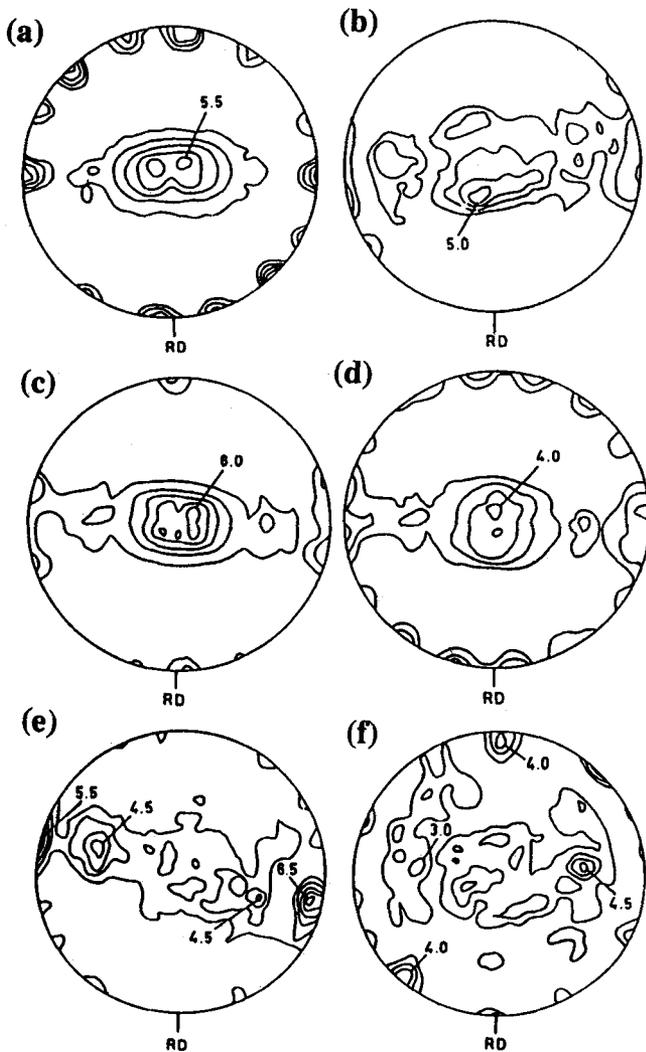
**Figure 5.** (0002) pole figures for the materials rolled at 1173 K (80%, furnace cooled), subjected to heat treatments at (a) 1173 K, (b) 1373 K; rolled at 1293 K (80%, furnace cooled), subjected to heat treatments at (c) 1173 K, (d) 1373 K; and rolled at 1373 K (80%, furnace cooled) subjected to heat treatments at (e) 1173 K, (f) 1373 K.
