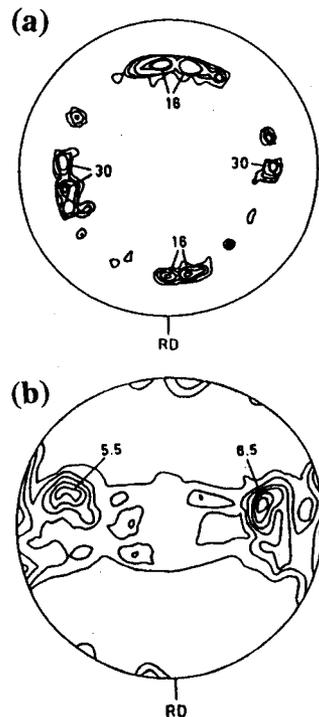
**Figure 3.** (a) (200) pole figure for the 1373 K rolled and water quenched material and (b) (0002) pole figure for the 1373 K rolled and furnace cooled material.
