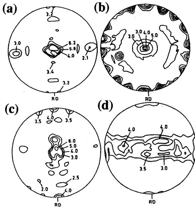
**Figure 1.** (0002) pole figures for the as-cast materials rolled at (a) 1173 K and water quenched, (b) 1173 K and furnace cooled, (c) 1293 K and water quenched and (d) 1293 K and furnace cooled.
