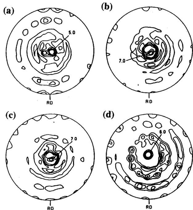
**Figure 4.** (0002) pole figures for the materials isothermally annealed at 1173 K for (a) 15 min, (b) 30 min, (c) 2 h and (d) 12 h.
