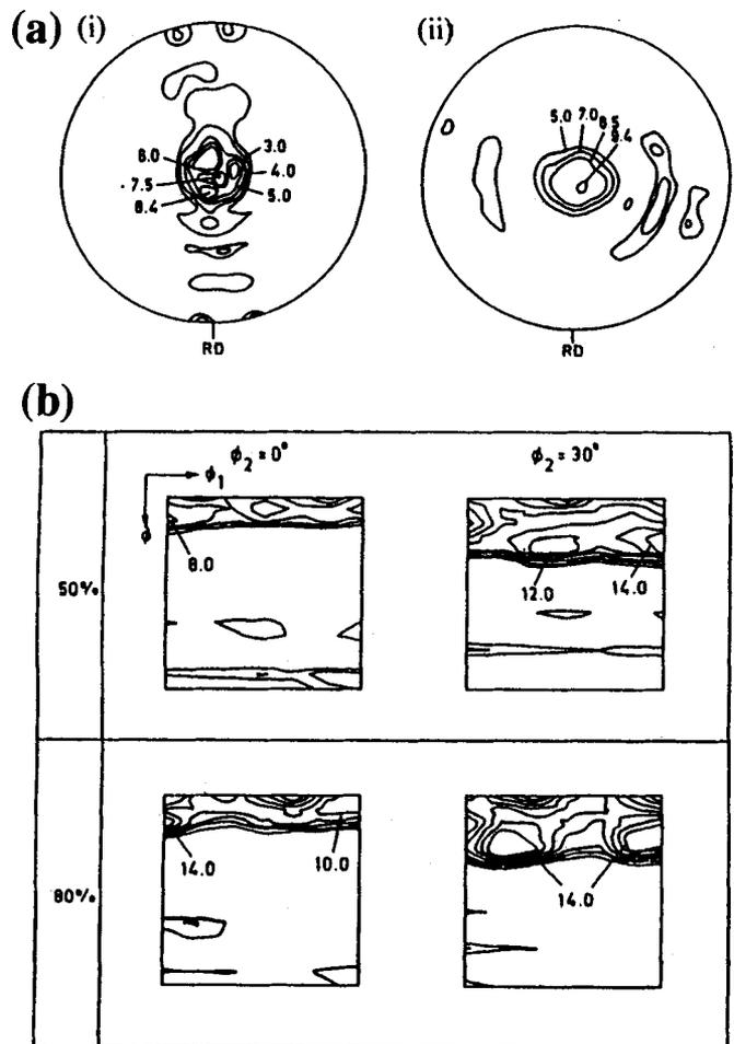
**Figure 2.** (a) (0002) pole figures for the material prior heat treated and rolled at 1173 K to the thickness reductions (i) 50% and (ii) 80% and (b)  $\phi_2 = 0^\circ$  and  $30^\circ$  sections of the ODFs for the same (50% and 80% rolled) materials.
