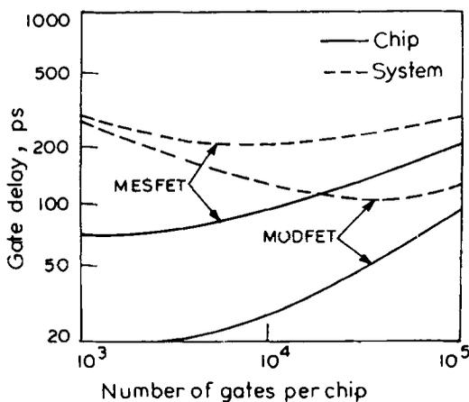
**Figure 4.** Propagation delay, whether measured on a chip or a system basis, will always be lower for MODFET than for MESFET. The optimum integration level for MODFET (the integration level yielding the lowest system delay) will be somewhere between 10,000 and 100,000 gates per chip. For purposes of comparison, power generation was set at 20 watts per square centimeter.
