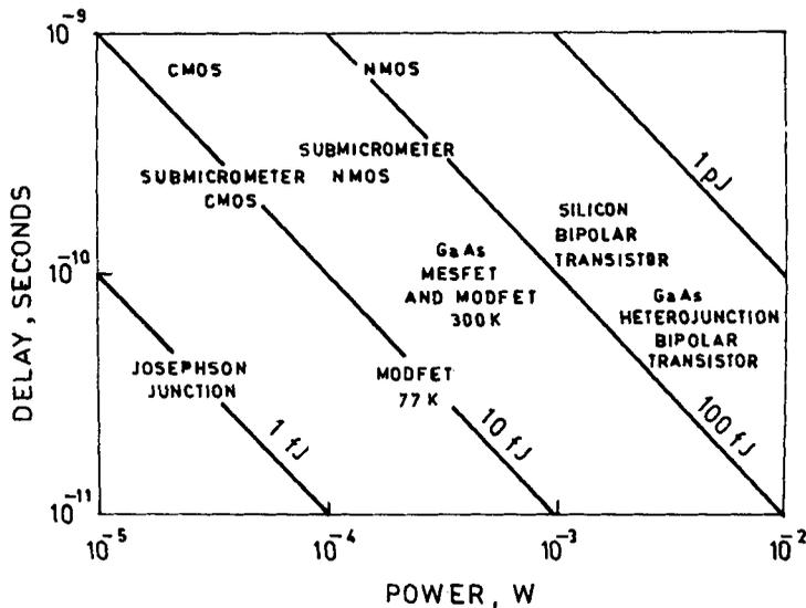
Figure 2. Power-delay continuums of important transistor technologies are indicated generally by circles, based on conservative design. The diagonal lines are lines of constant power-delay product. Only the Josephson junction offers comparable propagation delay and lower-power dissipation than the nitrogen-cooled (77 K) MODFET. The system-integration and -fabrication difficulties of the Josephson junction, however, appear insurmountable in the near future.
