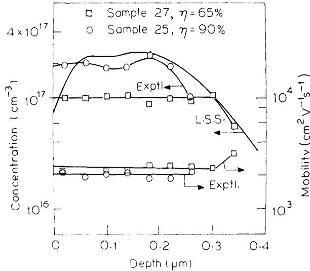
**Figure 1.** Electron concentration and mobility profiles obtained by differential Hall measurements at room temperature. The energies of  $^{29}\text{Si}^+$  are 60, 160 and 260 keV with doses of  $1 \times 10^{12}$ ,  $2.55 \times 10^{12}$  and  $3 \times 10^{12} \text{ cm}^{-2}$  respectively. The samples were thermally annealed at  $850^\circ\text{C}$  for 15 min in an  $\text{N}_2$  ambient with As overpressure.
