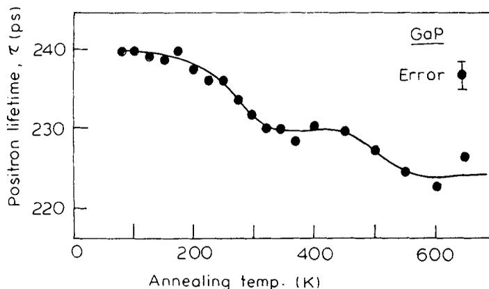
Figure 1. Variation in the positron lifetime in GaP with annealing temperature.
