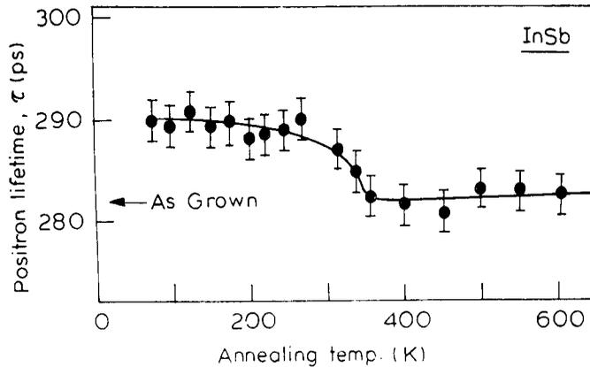
**Figure 2.** Variation in the positron lifetime in InSb during isochronal annealing treatment.
