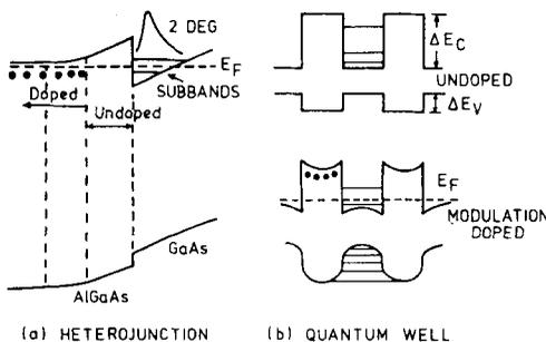
**Figure 2.** Band diagrams in (a) a heterojunction and (b) a quantum well.
