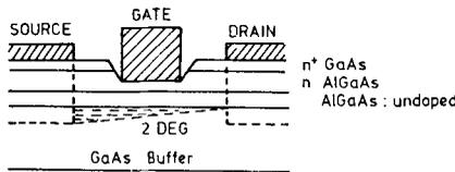
Figure 5. Cross-sectional view of an HEMT.
