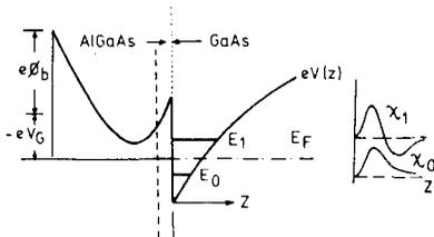
Figure 6. Band diagram in an HEMT for a positive gate voltage ( $V_g$ ).
