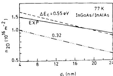
**Figure 8.** Variation of 2D carrier density versus spacer width ( $d_i$ ).
