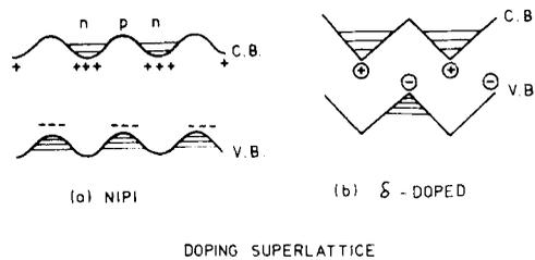
Figure 3. Band diagrams in (a) an NIPI and (b) a  $\delta$ -doped structure.
