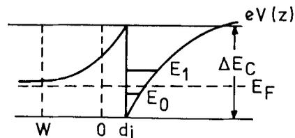
Figure 7. Band diagram in an HEMT under no gate bias.
