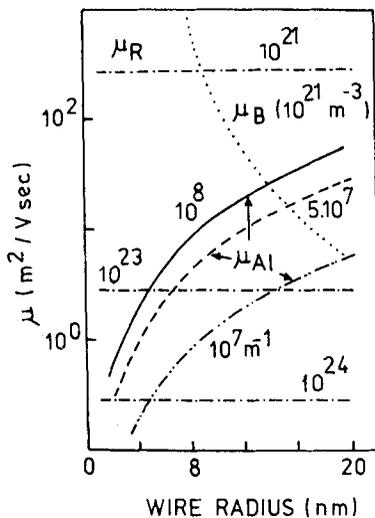
**Figure 9.** Alloy scattering limited mobility ( $\mu_{AL}$ ) in a 1D system for different IDEG densities.  $\mu_R$  and  $\mu_B$  denote respectively the remote impurity and background impurity scattering limited mobility.
