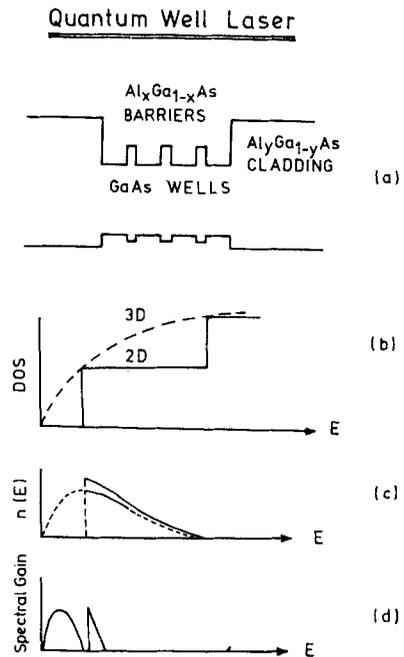
**Figure 10.** (a) Band diagram of a QW laser, (b) DOS function for bulk and 2D, (c) electron distribution as a function of energy, and (d) gain spectra.
