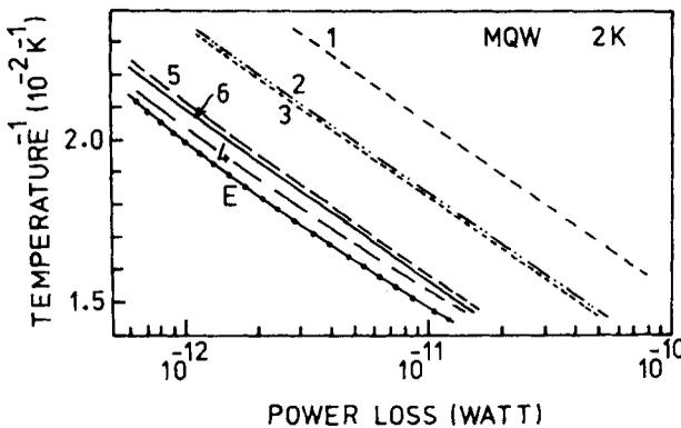
**Figure 11.** Power loss vs reciprocal electron temperature in a GaAs-AlGaAs MQW. E: experimental curve; 1: pure 2D; 2,3: phonon overlap function included; 4:  $q_s(0, 0, 0)$ ; 5:  $q_s(q, \omega_0, T_e)$ ; 6:  $q_s(q, \omega_0, T_e)$ , damping included.
