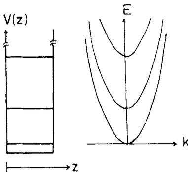
**Figure 1.** Quantisation of an electron in a narrow potential well, and formation of sub-bands. The  $E$ - $k$  relation is shown.
