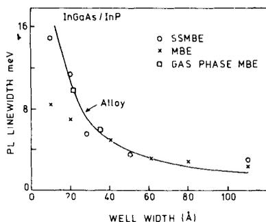
Figure 12. Photoluminescence linewidth (in meV) vs well width.
