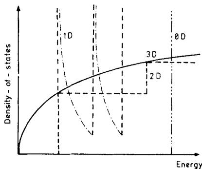
Figure 4. Density-of-states function for 3D, 2D, 1D and 0DEG.
