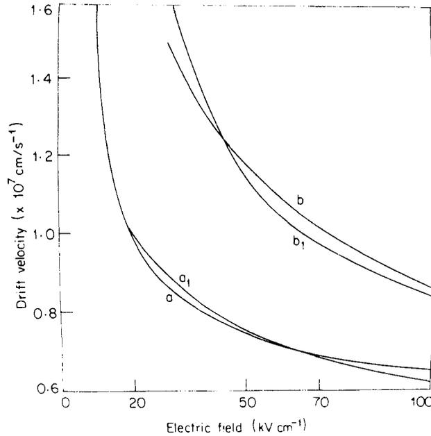
**Figure 1.** Velocity-field characteristics for bulk In (0.53) Ga (0.47) As at 300 K (a, a<sub>1</sub>) and 95 K (b, b<sub>1</sub>). a, b-theoretical, a<sub>1</sub>, b<sub>1</sub>-experimental.
