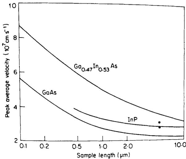
Figure 3. Peak average velocity in submicron samples for In (0.53) Ga (0.47) As, GaAs and InP.
