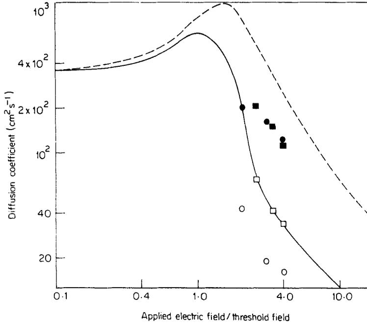
**Figure 2.** High-field transverse and parallel diffusion ( $D_{\perp}$ ,  $D_{\parallel}$ ) coefficients at 300 K for In (0.53) Ga(0.47)As, GaAs and InP. (Solid line— $D_{\parallel}$  for In(0.53)Ga(0.47)As; broken line— $D_{\perp}$  for In(0.53)Ga(0.47)As;  $\square$ — $D_{\parallel}$  for GaAs;  $\blacksquare$ — $D_{\perp}$  for GaAs;  $\circ$ — $D_{\parallel}$  for InP;  $\bullet$ — $D_{\perp}$  for InP.
