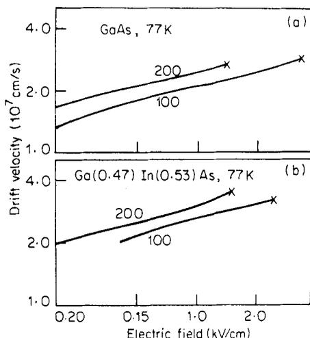
**Figure 4.** Velocity-field characteristics of In(0.53)Ga(0.47)As and GaAs in rectangular quantum wells for well widths of 100 and 200 Å.
