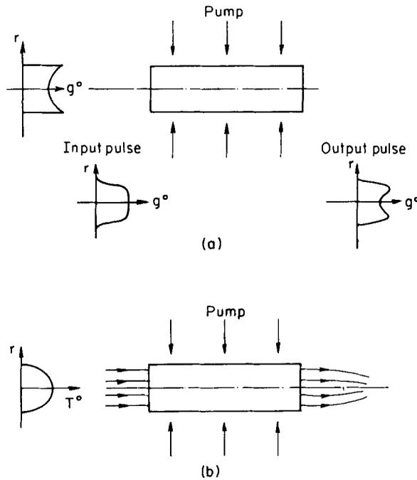
**Figure 1.** a. Gain variation in rod geometry—change in radial profile of beam. b. Temperature variation in rod geometry—thermal lensing.
