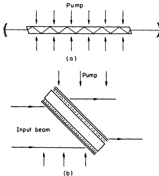
Figure 2. a. TIR slab geometry. b. Axial gradient configuration: disc amplifier geometry.
