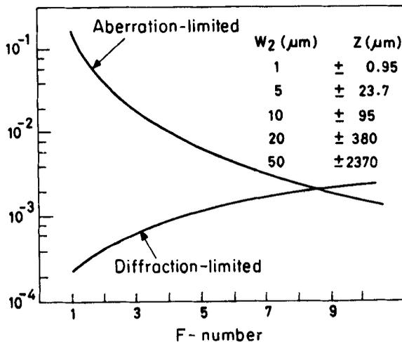
Figure 4. Focal spot size dependence on diffraction and lens aberration.
