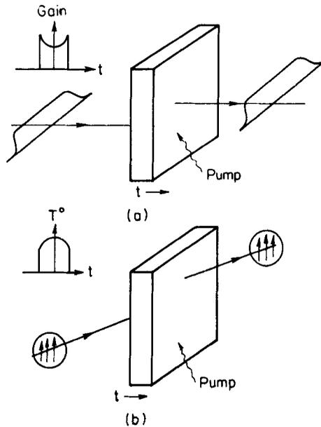
Figure 3. a. Gain variation in slab geometry and its effect on input beam. b. Polarization dependence due to one-dimensional temperature profile in disc geometry.
