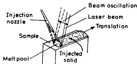
Figure 9. Schematic representation of laser melt particle injection process.
