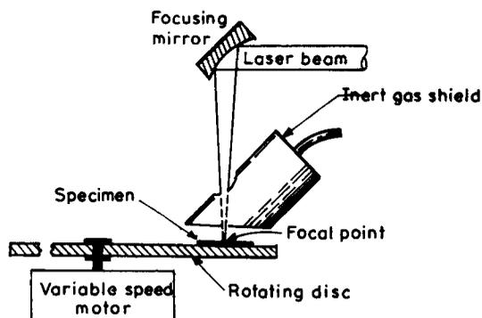
Figure 6. Schematic drawing of laser glazing process.
