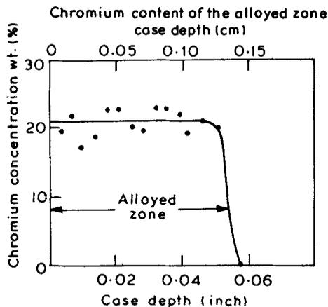
Figure 10. Chromium concentration in laser alloyed AISI 4815 steel.
