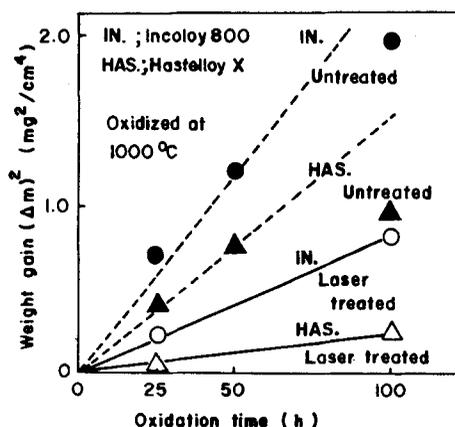
Figure 8. Oxidation behaviour of laser treated and untreated incoloy 800 and hastelloy X.
