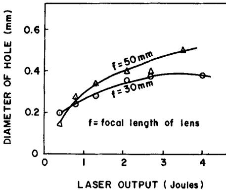
Figure 5. Diameter of hole as a function of lens focal length and laser power.
