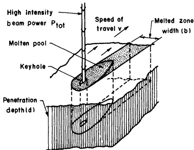
Figure 2. Keyhole mechanism.
