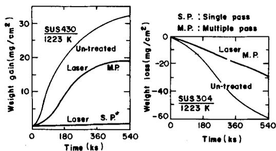
Figure 7. Changes in weight gain (loss) of the laser treated and untreated steels oxidized at 1223 K (calculated from thickness of oxide films).
