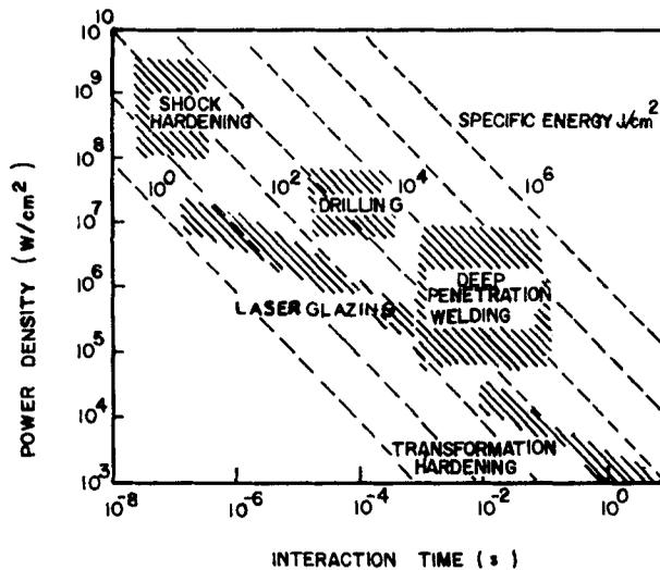
Figure 1. Process parameters for laser materials processing.
