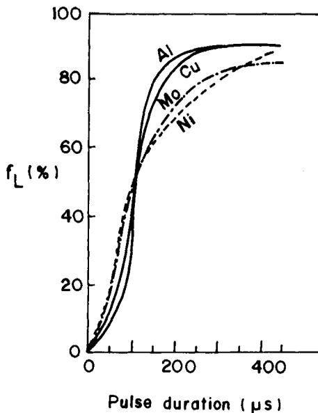
Figure 3. Material removed (%) in liquid phase as a function of laser pulse duration.
