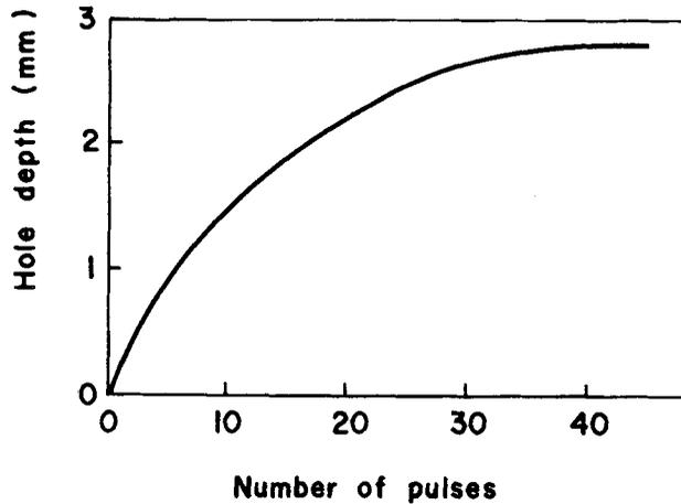
Figure 4. Effect of repeated pulsing on hole depth.
