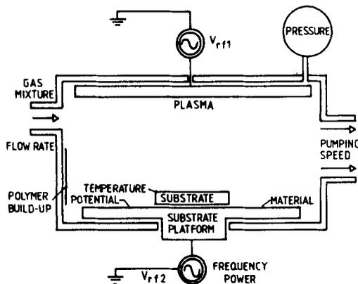
Figure 2. Schematic diagram of a parallel plate dry etching system.
