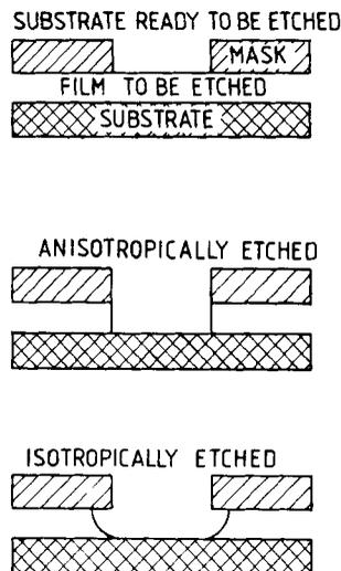
**Figure 1.** Isotropic and anisotropic etching of a masked thin film substrate.
