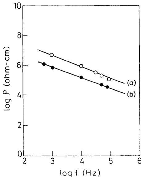
Figure 3. Plot of  $\log \rho_{ac}$  vs  $\log f$  for film of nominal composition  $Y_2GdFe_5O_{12}$  at temperatures a. 380° K and b. 650° K.
