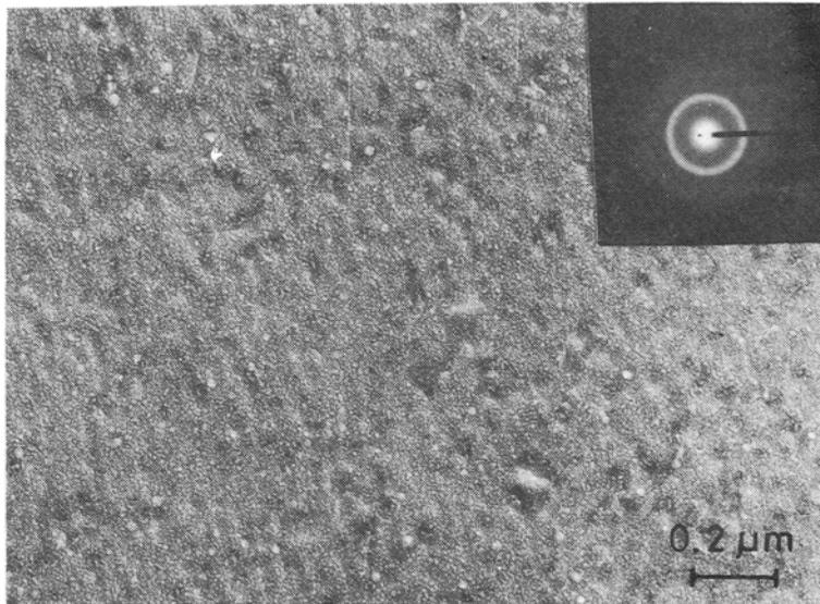
**Figure 1.** Electron micrograph of nominal composition Y<sub>2</sub>GdFe<sub>5</sub>O<sub>12</sub> heat-treated at 700°C for 1 hr. Inset shows the corresponding electron diffraction.
