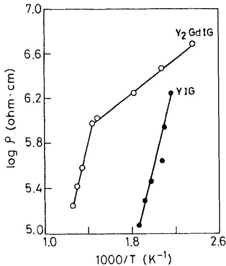
Figure 2. Plot of  $\log \rho_{dc}$  vs  $1000/T$  for films of nominal composition  $Y_3Fe_5O_{12}$  and  $Y_2GdFe_5O_{12}$ .
