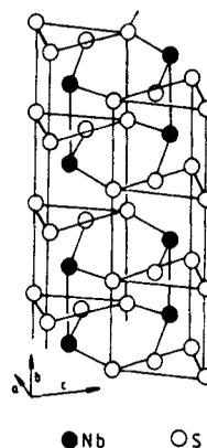
Figure 2. Structure of  $NbSe_3$ .
