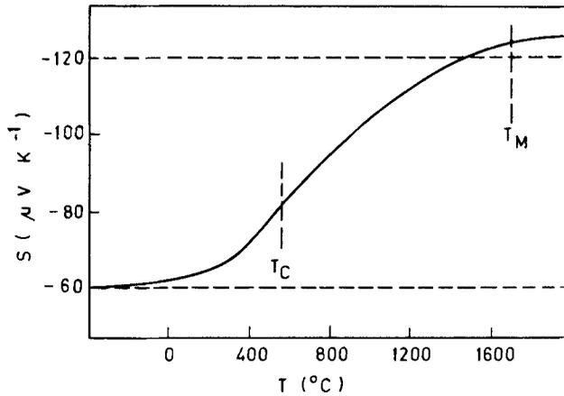
Figure 2. Thermoelectric power for the high temperature phase of magnetite (Wu and Mason 1981).
