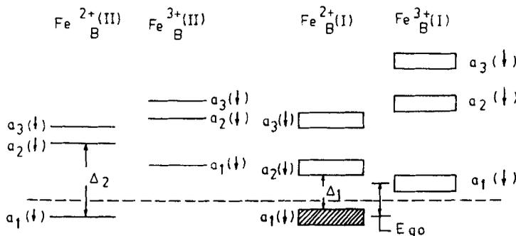
Figure 5. Splitting of  $\text{Fe}^{3+}/\text{Fe}^{2+}$  redox bands for  $T < T_v$  in the monoclinic phase of magnetite for the  $B$  site ions.
