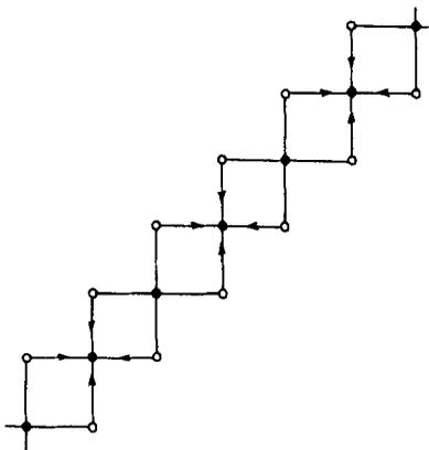
Figure 1. The active longitudinal optic mode of vibration responsible for the correlated electron transfer mechanism on the octahedral metal sites.
