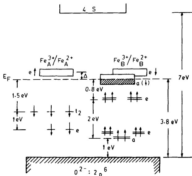
Figure 4. Electron energy band diagram of magnetite at room temperature (Goodenough 1982).
