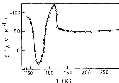
Figure 3. Thermoelectric power for the low temperature phase of magnetite (Graener *et al* 1979).
