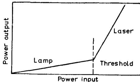
Figure 2. Power output vs. input in a laser which shows that beyond a certain value of the input power, laser light becomes coherent.
