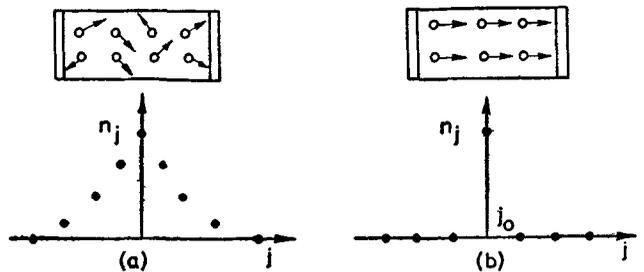
Figure 6. Photon selection in a laser with two end mirrors.
