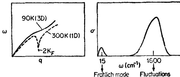
Figure 3 (b). The a.c. conductivity of  $\text{K}_2\text{Pt}(\text{CN})_4 \text{Br}_{0.3}$ .
