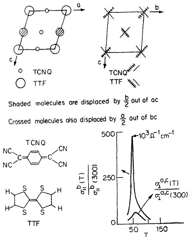
Figure 2. Crystal structure and conductivity of TTF-TCNQ.
