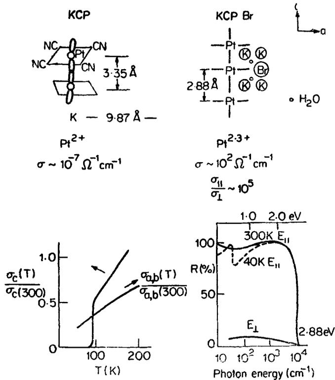
Figure 3 (a). The metal chain complex  $\text{K}_2\text{Pt}(\text{CN})_4$  and  $\text{K}_2\text{Pt}(\text{CN})_4\text{Br}_{0.3}$ : crystal structure, conductivity and reflectivity data.
