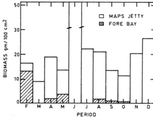
**Figure 6.** Seasonal variation in fouling biomass in coastal waters (MJ) and forebay (FB) during 1986-87. Data represent wet weight in g/100 cm<sup>2</sup> from short term panels.
