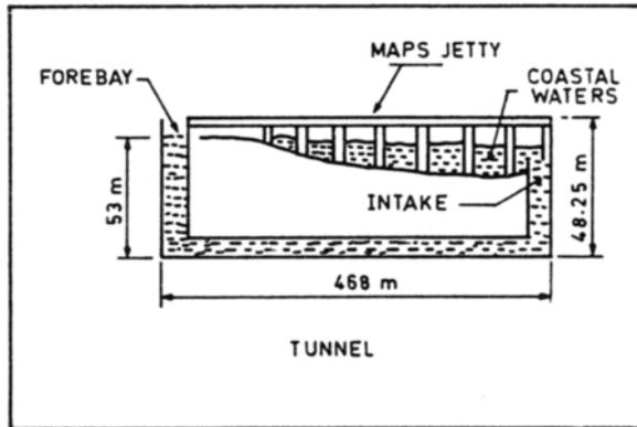
Figure 1. A schematic view of MAPS seawater tunnel.
